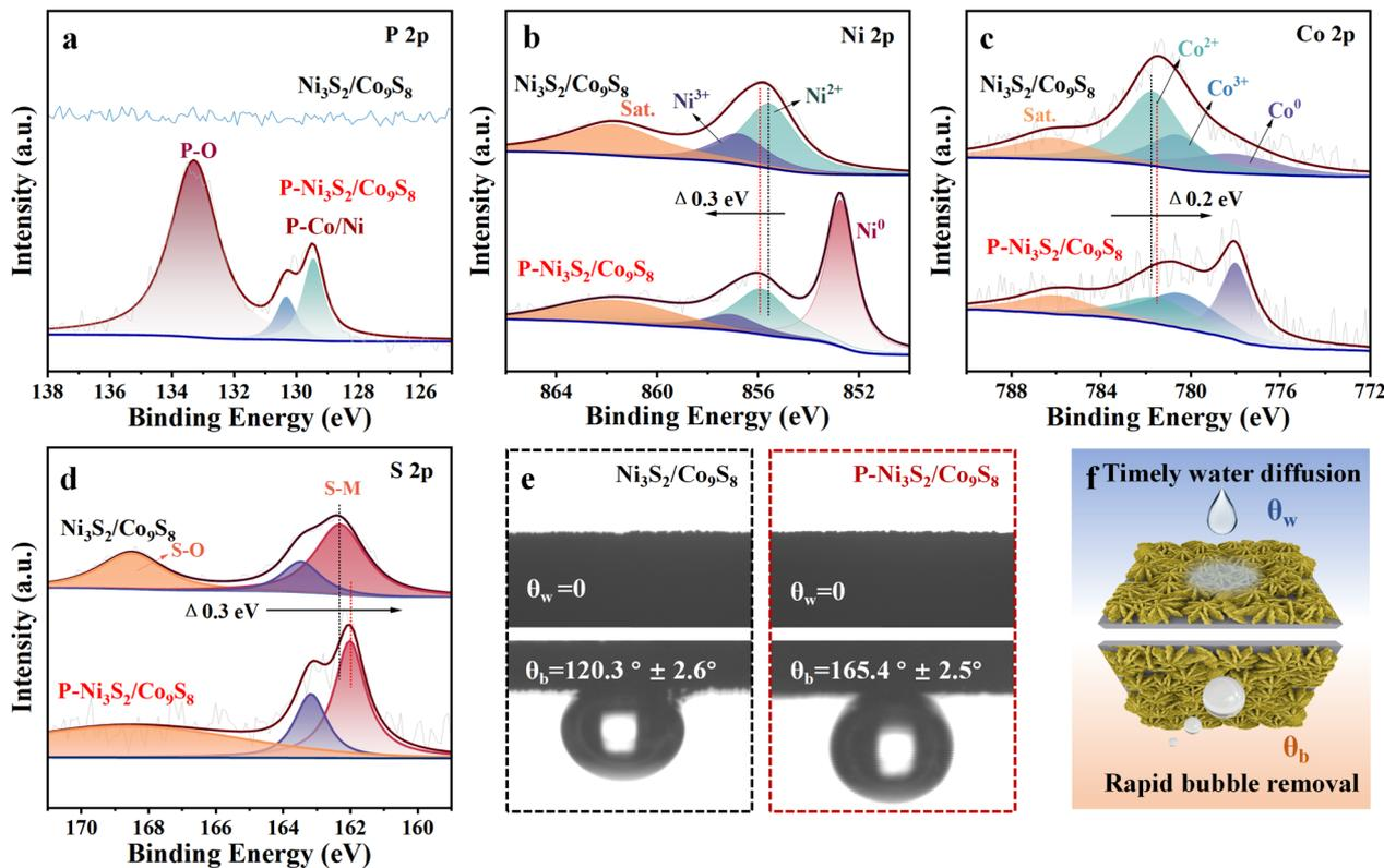
Fig. 2 XPS spectra of (a) P 2p, (b) Ni 2p, (c) Co 2p and (d) S 2p for  $\text{Ni}_3\text{S}_2/\text{Co}_9\text{S}_8$  and  $\text{P-Ni}_3\text{S}_2/\text{Co}_9\text{S}_8$ . (e) Static water/bubble contact angle images of  $\text{Ni}_3\text{S}_2/\text{Co}_9\text{S}_8$  and  $\text{P-Ni}_3\text{S}_2/\text{Co}_9\text{S}_8$ . (f) Schematic illustration of the superhydrophilic and superaerophobic properties of  $\text{P-Ni}_3\text{S}_2/\text{Co}_9\text{S}_8$ .
