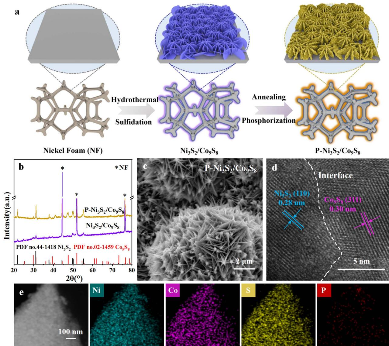
Fig. 1 (a) Schematic illustration of the synthetic procedure of P-Ni<sub>3</sub>S<sub>2</sub>/Co<sub>9</sub>S<sub>8</sub>. (b) XRD patterns of Ni<sub>3</sub>S<sub>2</sub>/Co<sub>9</sub>S<sub>8</sub> and P-Ni<sub>3</sub>S<sub>2</sub>/Co<sub>9</sub>S<sub>8</sub>. (c) SEM image, (d) HRTEM image, and (e) HAADF-STEM image with the corresponding energy-dispersive spectrometry (EDS) mapping images of P-Ni<sub>3</sub>S<sub>2</sub>/Co<sub>9</sub>S<sub>8</sub>.
