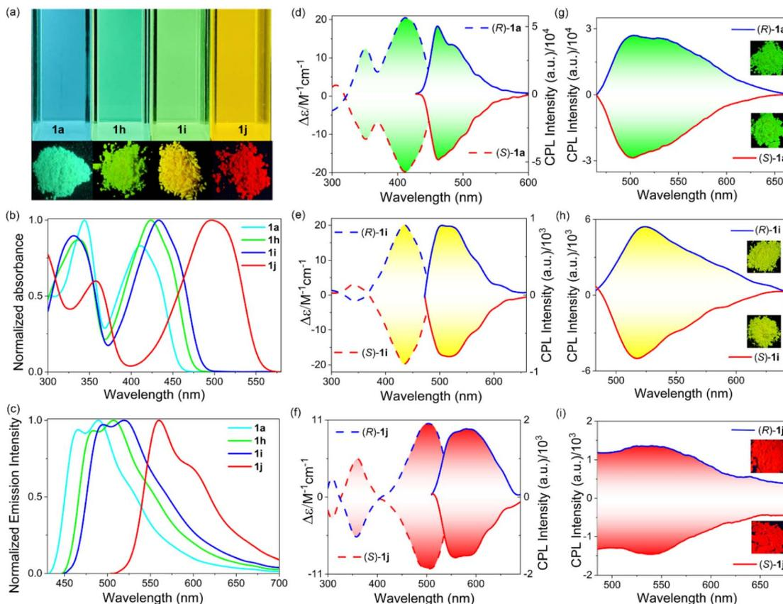
Fig. 3 Photophysical and chiroptical properties of **1a** and **1h–j** in dichloromethane and solid states. (a) Fluorescence photos of respective **1a** and **1h–j** taken under a 365 nm lamp. (b) Normalized UV-vis absorption and (c) emission spectra in dichloromethane. (d)–(f) CD (dash lines) and CPL spectra (solid lines) of (S/R)-**1a** (d) and (g), **1i** (e) and (h), and **1j** (f) and (i) in dichloromethane and solid states.
