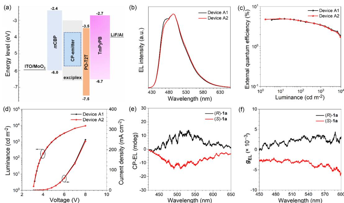
Fig. 5 (a) Configuration diagram of the fabricated devices. (b) EL spectra measured at  $1000 \text{ cd m}^{-2}$ , (c) external quantum efficiency curves with the change of luminance, and (d) luminance and current density curves with the change of voltage of devices A1 and A2. (e) CPEL spectra were collected under 5 V and (f) plots of  $g_{\text{EL}}$  versus CP-EL wavelength of devices A1 and A2.
