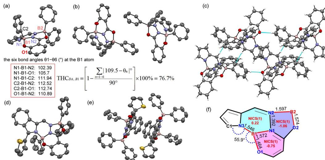
Fig. 2 (a)–(c) X-ray crystal, dimer, and packing structures of **1a**. (d) and (e) X-ray crystal and dimer structures of **1j**. (f) NICS(1) values for **1a**. Peripheral substituents and hydrogen atoms were removed for clarity. Thermal ellipsoids are shown at the 50% probability level. Selected bond lengths in **1a**: B1–N1, 1.572 Å; B1–N3, 1.545 Å; B2–N2, 1.597 Å; B1–O1, 1.464 Å; B2–O2, 1.574 Å. C, gray; N, light blue; B, pink; O, red; S, yellow.
