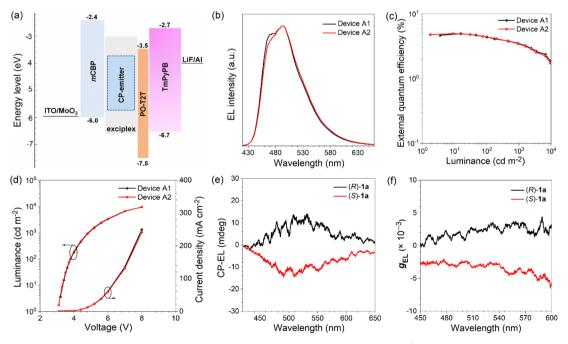
Fig. 5 (a) Configuration diagram of the fabricated devices. (b) EL spectra measured at 1000 cd m $^{-2}$ , (c) external quantum efficiency curves with the change of luminance, and (d) luminance and current density curves with the change of voltage of devices A1 and A2. (e) CPEL spectra were collected under 5 V and (f) plots of  $g_{EL}$  versus CP-EL wavelength of devices A1 and A2.
