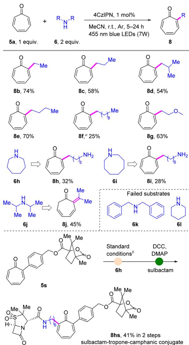
**Scheme 3** Scope of symmetric secondary amines for  $\alpha$ -alkylation of tropones. Reaction conditions: entry 1 in Table 1, irradiation time = 5–24 h. See the ESI† for details. Isolated yields are reported.<sup>a</sup> 0.283 mmol troponone (**5a**) and 0.283 mmol diethylamine (**6f**) were used due to the poor solubility of **6f** in MeCN.<sup>b</sup> 0.1 mmol **5s** and 0.1 mmol azocane (**6h**) were used. DCC = *N,N'*-dicyclohexylcarbodiimide and DMAP = 4-dimethylaminopyridine.
