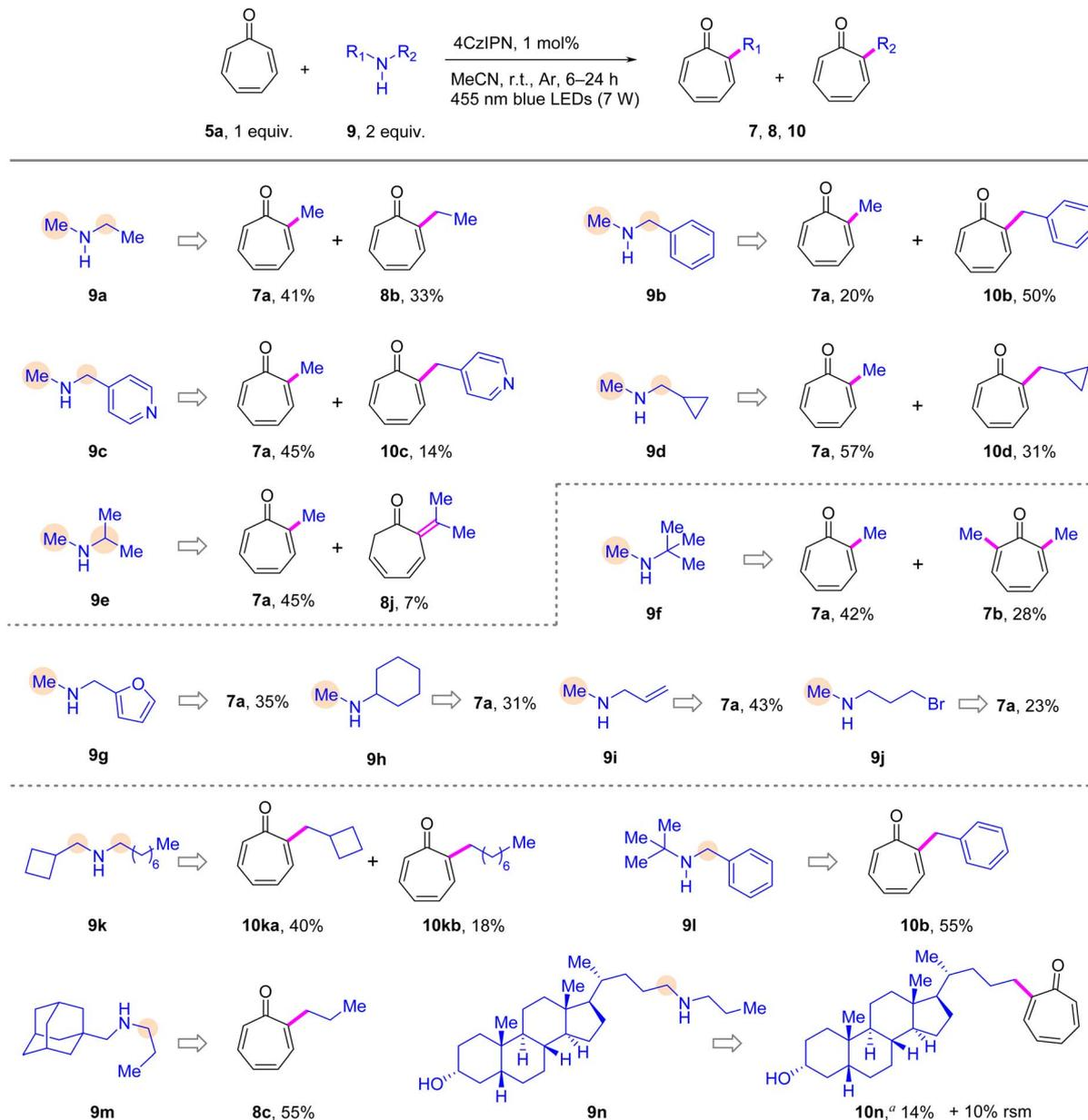
Scheme 4 Scope of asymmetric secondary amines for  $\alpha$ -alkylation of tropones. Reaction conditions: entry 1 in Table 1, irradiation time = 6–24 h. See the ESI† for details. Isolated yields are reported.<sup>a</sup> 0.849 mmol **5a** and 0.283 mmol **9n** were used in MeCN/THF/DCM (5.7 mL/0.57 mL/1.2 mL). rsm = recovered starting material.
