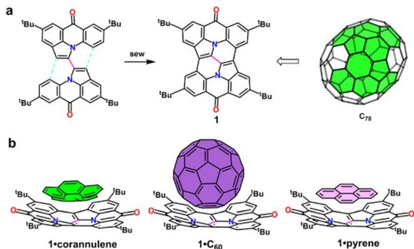
Fig. 1 (a) The nitrogen-containing buckybowl **1**, synthesized using a core-periphery strategy featuring a single-bond core, can be considered as an aza-analogue of a C<sub>78</sub> fullerene fragment. (b) Schematic representation of the interactions between **1** and corannulene, C<sub>60</sub>, or pyrene.
