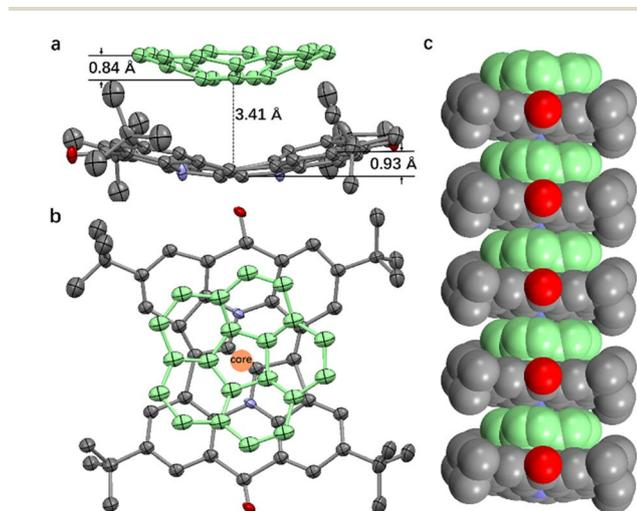
Fig. 5 (a) ORTEP diagram of the **1**·corannulene complex, with thermal ellipsoids shown at the 30% probability level. (b) Overlay of the core structures of compound **1** and corannulene within the single-crystal structure of **1**·corannulene. (c) One-dimensional self-assembled structure formed by compound **1** and corannulene. Corannulene is depicted in green, and hydrogen atoms are omitted for clarity.
