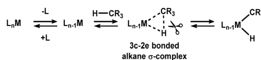
Scheme 1 An illustration of how coordinatively unsaturated metal complexes and C–H bonds can interact to form a 3-centre 2-electron (3c-2e) \sigma -complex prior to the oxidative cleavage of the C–H bond.
