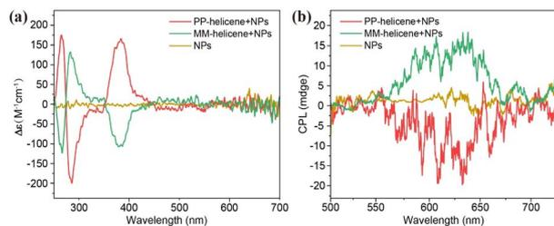
**Fig. 2** (a) Circular dichroism spectra of NPs, (*P,P*)-helicene + NPs, and (*M,M*)-helicene + NPs in dichloromethane. (b) Upconversion CPL spectra of NPs, (*P,P*)-helicene + NPs and (*M,M*)-helicene + NPs in dichloromethane ( $\lambda_{\text{ex}} = 980$  nm).
