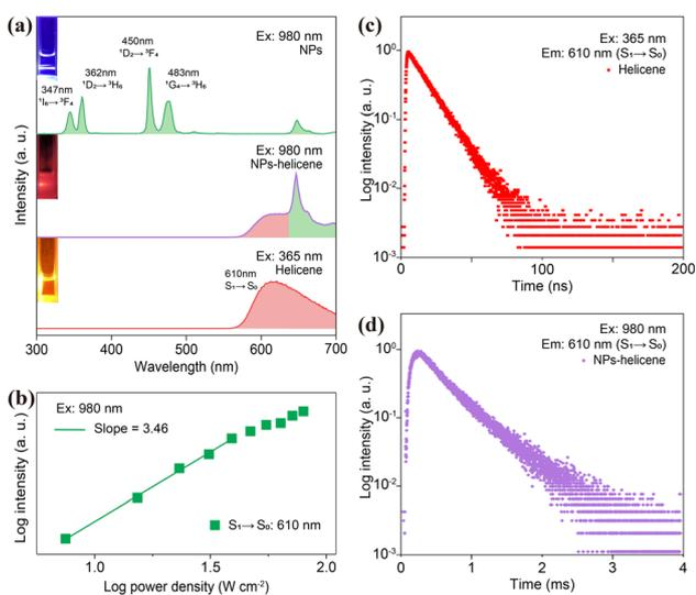
**Fig. 1** (a) PL spectrum of helicene under 365 nm excitation, and UCL spectra of the NPs (green) and NPs-helicene (purple) under 980 nm excitation at a power density of 22 W cm<sup>-2</sup>. (b) Power density dependence of NPs-helicene at 610 nm, indicating a four-photon population process. (c) PL decay curves of helicene at 610 nm under 365 nm excitation. (d) UCL decay curves of NPs-helicene at 610 nm under 980 nm excitation.
