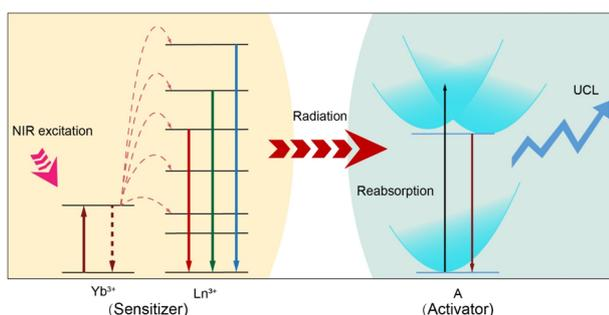
**Scheme 1** Schematic illustration of the radiative energy transfer upconversion processes in various optical nanomaterials (activator: A = chiroptical materials, transition metal complexes, lanthanide complexes, metal nanoclusters, conjugated polymers, nanoscale carbon allotropes, fluorescent dyes, and quantum dots) through lanthanide-doped nanoparticle (sensitizer) sensitization.
