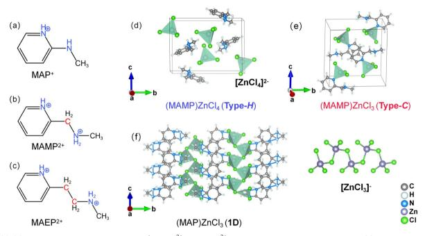
Fig. 1 (a)-(c) Protonated organic compounds MAP+, MAMP<sup>2+</sup>, and MAEP<sup>2+</sup>, with steric hindrance highlighted in red; (d) representative Type-H compound (MAMP)ZnCl<sub>4</sub>; (e) representative Type-C compound (MAMP)ZnCl<sub>3</sub>; (f) rare 1D zinc-based compound (MAP)ZnCl<sub>3</sub>, with an enlarged view of its inorganic 1D chain.
