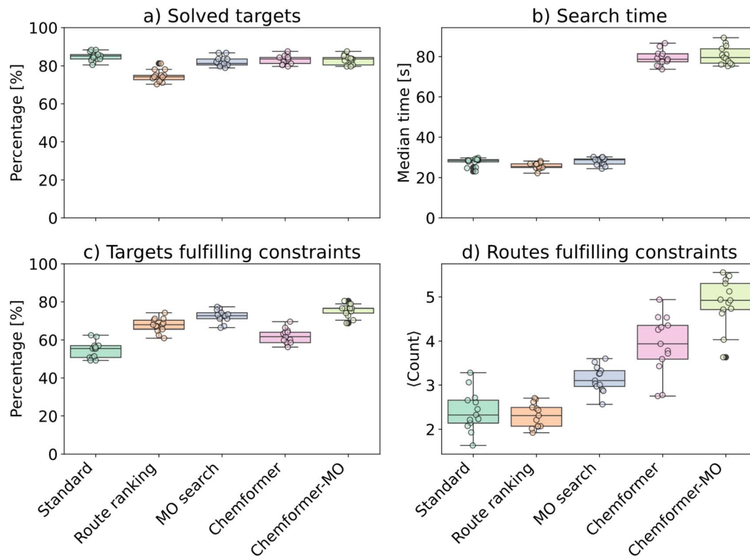
Fig. 2 Performance of the different disconnection-aware strategies with standard search as the baseline. Performance is measured in terms of (a) percentage of solved targets, (b) median search time, (c) percentage of targets which are solved and fulfill the bond constraints and (d) average number of routes which are solved and fulfill the bond constraints. The full PaRoutes set-n1 targets were divided into batches with batch size 128 in order to facilitate statistics calculations (Methods; "Statistical variation from batches"). Each colored dot corresponds to one batch. Box-plot elements: center line is the median, box limits are the upper and lower quartiles, whiskers are 1.5 times the interquartile range, and outliers are depicted as black dots.
