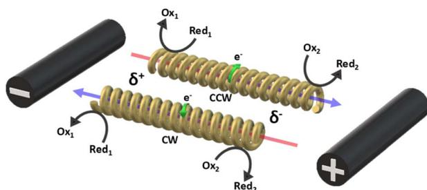
**Scheme 1** Illustration of the current produced by the wirelessly triggered redox reactions taking place at the extremities of a clockwise or anticlockwise solenoid, with a representation of the currents produced by the chemical reactions and the exogenous chemically-induced magnetic field. The blue and red colored arrows represent the north and south pole of the generated magnetic fields, respectively.
