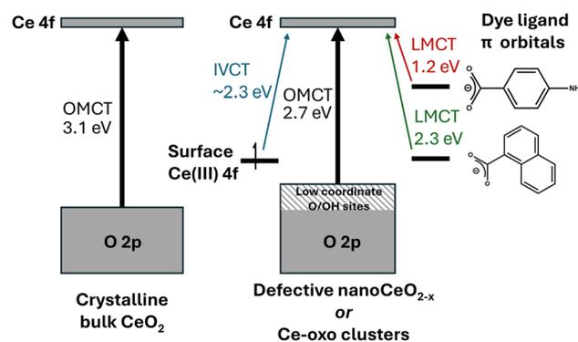
Fig. 9 Diagram proposing the major contributions to the absorption spectra of  $\text{CeO}_2$  and (dye-sensitised) mixed valence Ce-oxo clusters. Note that dye ligands may also contribute to LUMO position.
