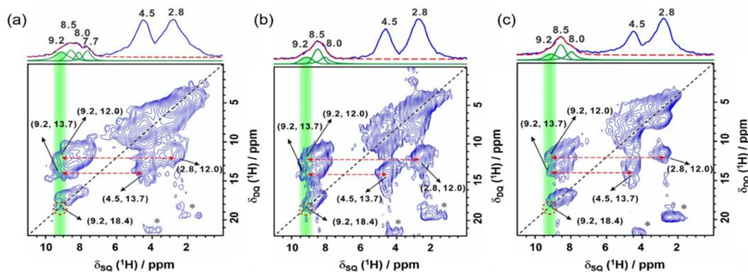
Fig. 3  $^1\text{H}$  DQ–SQ MAS NMR spectra of as-synthesized (a) 134TMP-PWO, (b) 135TMP-PWW and (c) 123TMP-RTH. The interactions between  $\text{SiO}^-$  and two SiOH groups and between these defects and TMP cations are indicated by red dashed circles and lines, respectively. Deconvolution of the bands centered at 8.5 ppm was done by considering  $^1\text{H}$  NMR resonances of the TMP cations in  $\text{D}_2\text{O}$ . Artifacts from the rotor and probe background are marked by asterisks.
