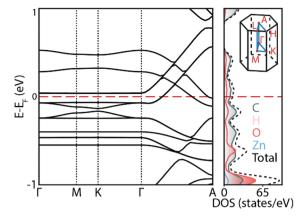
Fig. 3 Calculated band structure with projected density of states (DOS) of  $Zn_3(HOTP)_2$ . The inset shows the first Brillouin zone of the material with high symmetry k-points.  $Zn_3(HOTP)_2$  has a small band gap in the in-plane direction, and significant band curvature is observed in the out-of-plane direction.  $Zn_3(HOTP)_2$  is calculated to be metallic, as demonstrated by the band crossing the Fermi-level in the out-of-plane direction, and a non-zero projected DOS at the Fermi-level
