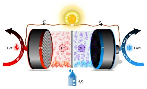
Scheme 1 Schematic diagram of electrochemical water formation assisted galvanic-thermogalvanic device for waste heat recovery.
