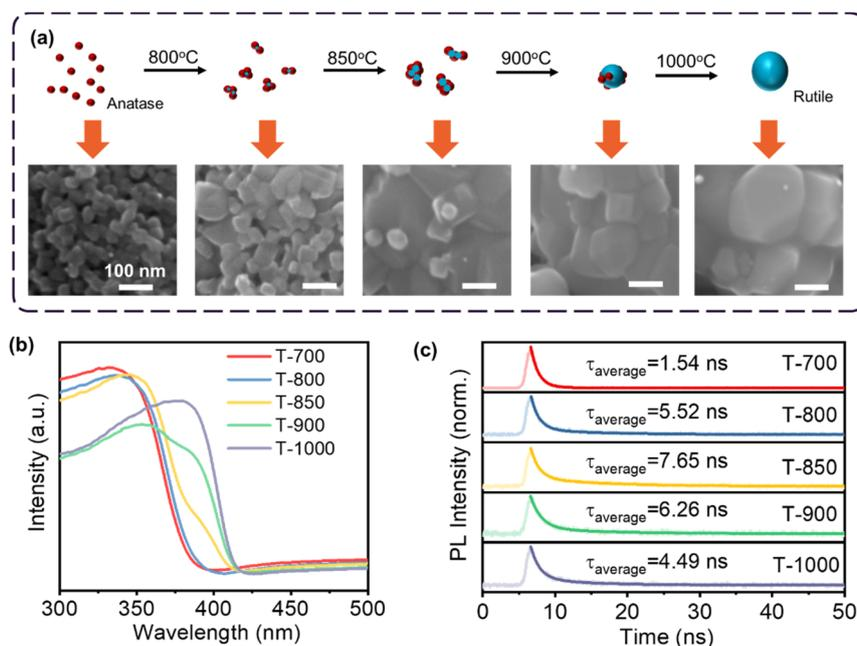
Fig. 2 (a) Schematic illustration of TiO<sub>2</sub> particle growth with the corresponding SEM images; (b) UV-vis spectra of commercial anatase annealed at different temperatures having different ratios of the rutile phase; (c) the TRPL decay curves of the as-prepared TiO<sub>2</sub> photocatalysts.
