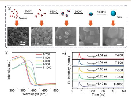
Fig. 2 (a) Schematic illustration of  $TiO_2$  particle growth with the corresponding SEM images; (b) UV-vis spectra of commercial anatase annealed at different temperatures having different ratios of the rutile phase; (c) the TRPL decay curves of the as-prepared  $TiO_2$  photocatalysts.
