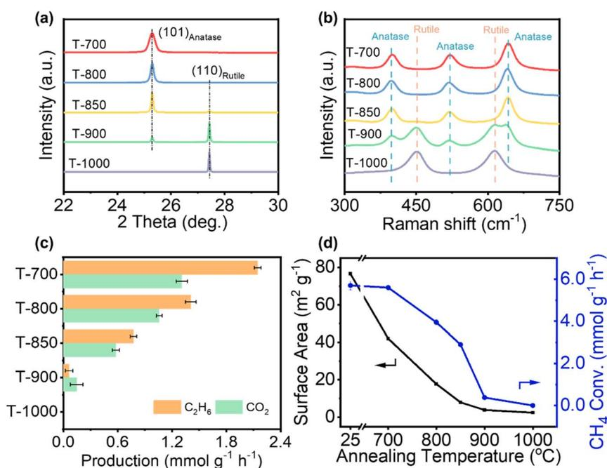
Fig. 1 The change in the TiO<sub>2</sub> photocatalyst at different temperatures (from 700 °C to 1000 °C), as determined from (a) XRD patterns and (b) Raman spectra. (c) POCM performance of different TiO<sub>2</sub>-based photocatalysts (orange bar: C<sub>2</sub>H<sub>6</sub>; green bar: CO<sub>2</sub>). (d) The CH<sub>4</sub> conversion rate (blue dot line) and the surface area change (black dot line) of different TiO<sub>2</sub>-based photocatalysts prepared at different temperatures.
