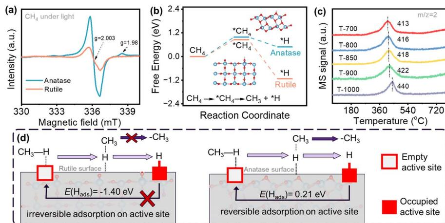
Fig. 4 (a) *In situ* EPR spectra of anatase and rutile; (b) computed Gibbs free energy of methane activation steps on anatase (101) and rutile (110) surfaces; (c) TPD-CH<sub>4</sub>-MS spectra of as-prepared TiO<sub>2</sub> photocatalysts; (d) schematic illustration of surface adsorption behaviour of CH<sub>4</sub> on rutile and anatase, respectively.
