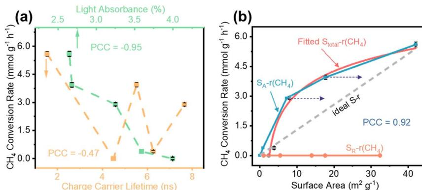
Fig. 3 CH<sub>4</sub> conversion rate ( $r(\text{CH}_4)$ ) plotted against (a) the charge carrier lifetime (orange) and light absorbance (green) and (b) surface area.
