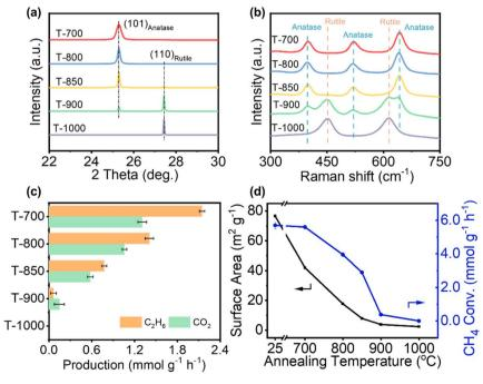
Fig. 1 The change in the  $TiO_2$  photocatalyst at different temperatures (from 700 °C to 1000 °C), as determined from (a) XRD patterns and (b) Raman spectra. (c) POCM performance of different  $TiO_2$ -based photocatalysts (orange bar:  $C_2H_6$ ; green bar:  $CO_2$ ). (d) The  $CH_4$  conversion rate (blue dot line) and the surface area change (black dot line) of different  $TiO_2$ -based photocatalysts prepared at different temperatures.
