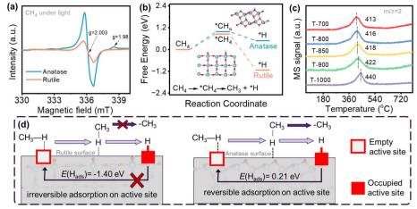
Fig. 4 (a) In situ EPR spectra of anatase and rutile; (b) computed Gibbs free energy of methane activation steps on anatase (101) and rutile (110) surfaces; (c) TPD-CH<sub>4</sub>-MS spectra of as-prepared  $TiO_2$  photocatalysts; (d) schematic illustration of surface adsorption behaviour of CH<sub>4</sub> on rutile and anatase, respectively.
