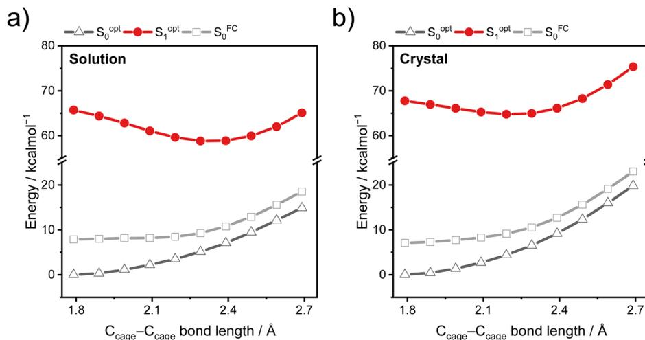
Fig. 5 Energy levels of the  $S_0$  and  $S_1$  states of H-H with variable  $C_{\text{cage}}-C_{\text{cage}}$  bond lengths in the (a) solution state and (b) crystalline state.  $S_0^{\text{opt}}$  and  $S_1^{\text{opt}}$  denote energy levels of optimized geometries in ground state and excited state, respectively.  $S_0^{\text{FC}}$  denotes energy levels calculated with single-point energy calculation using  $S_1$  excited-state optimized geometries.
