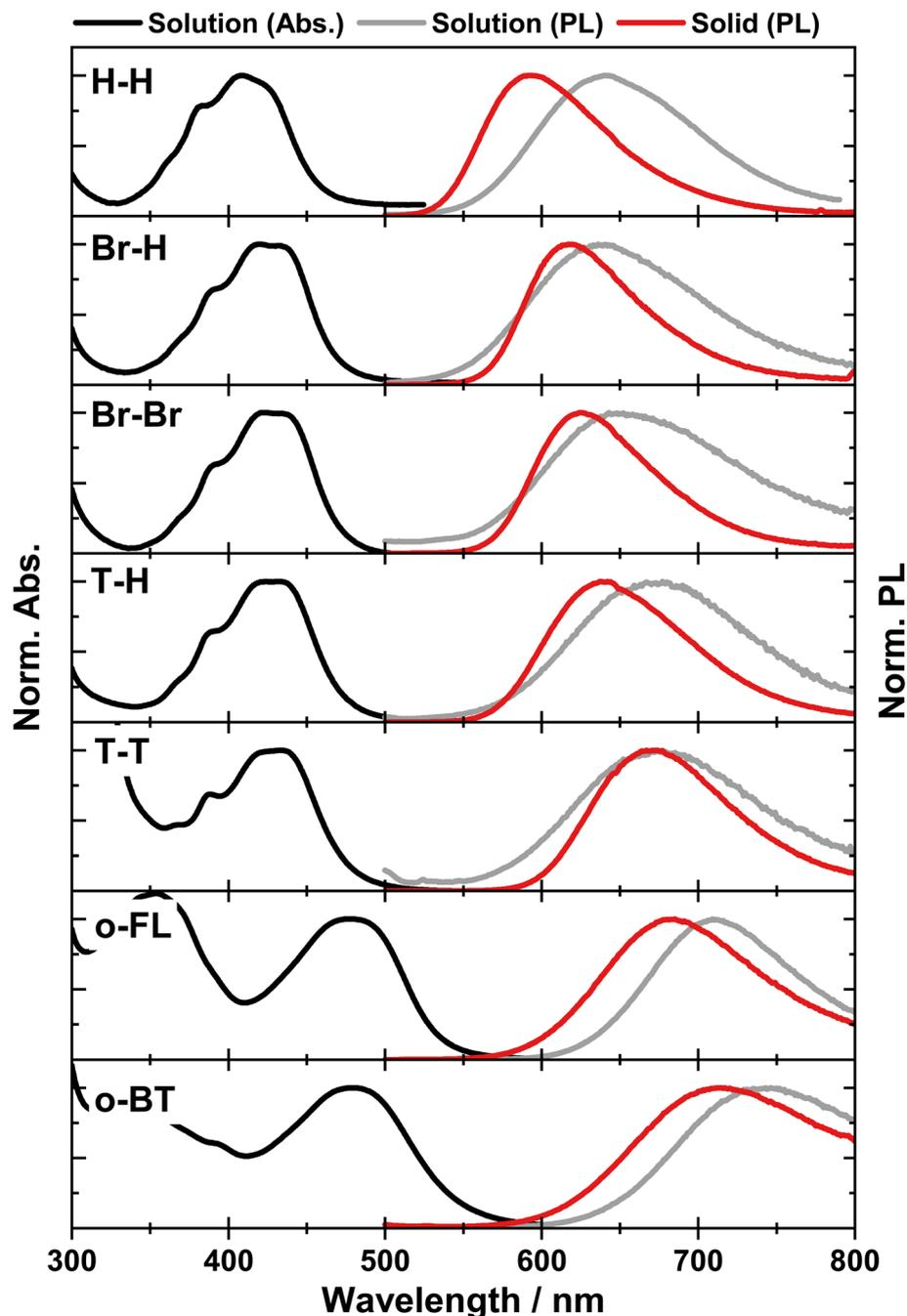
Fig. 2 Normalized UV-visible absorption (Abs.) and photoluminescence (PL) spectra of *C,C'*-diaryl-*o*-carborane derivatives (solution: chloroform,  $1.0 \times 10^{-5}$  M).
