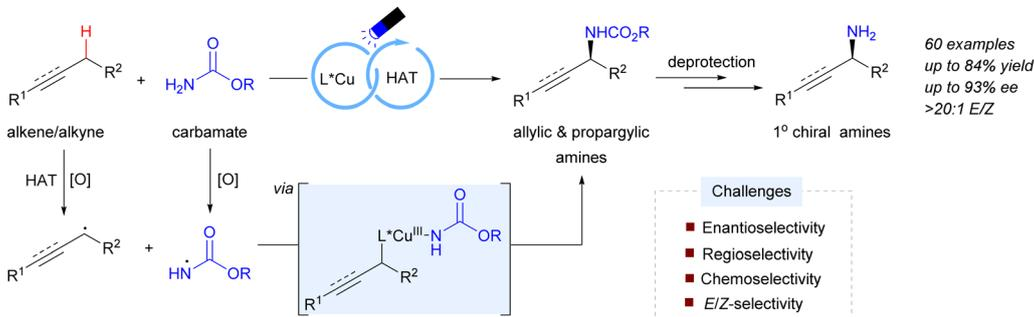
Scheme 1 Catalytic asymmetric allylic C–H amination reactions.
