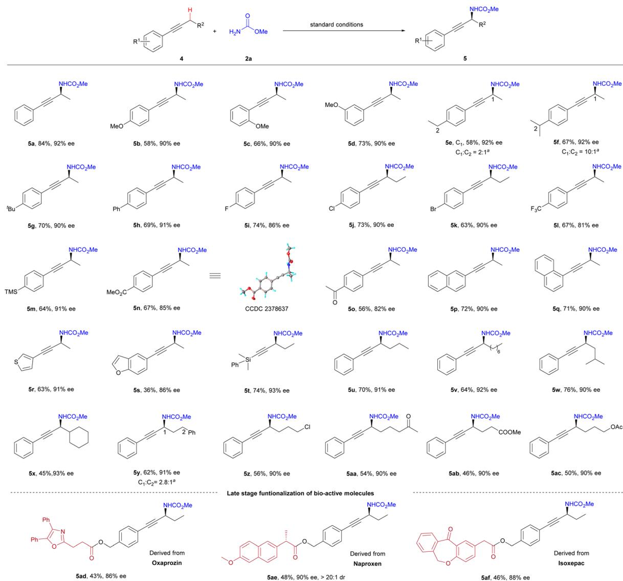
Scheme 3 Substrate scope of alkynes. Isolated yield, ee values were determined by chiral HPLC. <sup>a</sup>The ratio of site-isomers was determined by <sup>1</sup>H NMR.
