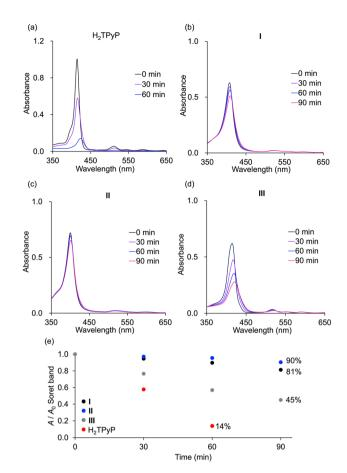
Fig. 7 Time-dependent absorption spectra of (a)  $H_2$ TPyP and (b) hybrid I, (c) hybrid II, and (d) hybrid III in acetonitrile/dichloromethane (1/1, v/v) upon photoirradiation ( $\lambda$  > 350 nm) in air. (e) Changes in the  $A/A_0$  values of the Soret band of hybrids I, II, and III and  $H_2$ TPyP (A: Soret band intensity;  $A_0$ : initial Soret band intensity).
