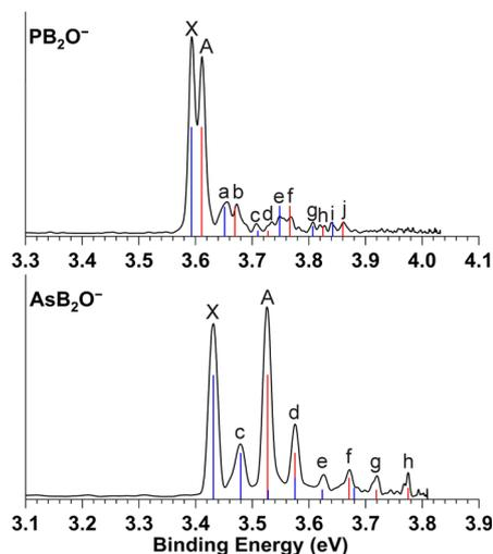
Fig. 4 Comparison of the calculated Franck–Condon factors (vertical lines) with the PE spectra of  $\text{PB}_2\text{O}^-$  at 4.032 eV and  $\text{AsB}_2\text{O}^-$  at 3.809 eV. The blue and red colours represent the Franck–Condon factors of the  $^2\Pi_{3/2}$  and  $^2\Pi_{1/2}$  states, respectively.
