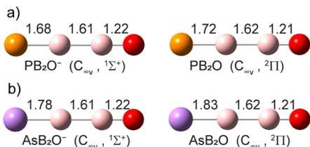
Fig. 3 The optimized structures of  $\text{PB}_2\text{O}^-$  and  $\text{AsB}_2\text{O}^-$  and the corresponding neutrals at the B3LYP/6-311+G\* level. The point group symmetries and electronic states are also given. The bond lengths are given in Å.
