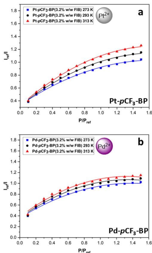
Fig. 7 The modified Stern–Volmer calibrated luminescent response to pressure with 2nd order polynomial fits (eqn (S2)†) at 273 K, 293 K and 313 K for (a) **Pt-pCF<sub>3</sub>-BP**(3.2% w/w FIB) (average  $R^2 = 0.995$ ). (b) **Pd-pCF<sub>3</sub>-BP**(3.2% w/w FIB) (average  $R^2 = 0.980$ ). The average  $R^2$  is across the fits for the three temperatures.
