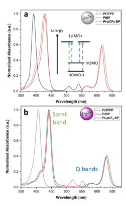
Fig. 2 The UV-Vis electronic absorption spectra of (a) PtTFPP,<sup>32</sup> PtBP and Pt-pCF<sub>3</sub>-BP and (b) PdTFPP,<sup>33</sup> PdBP and Pd-pCF<sub>3</sub>-BP in chloroform. Accompanying this, is a typical energy level diagrams showing the four frontier MOs found in tetraphenyl porphyrins and the electronic transitions that form the Soret and Q band features.
