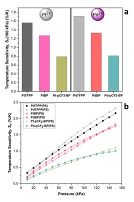
Fig. 6 (a) The  $S_T$  at 100 kPa,  $S_T$ (100 kPa) for the polystyrene-based PSPs. (b) The change in  $S_T$  with pressure for PtTFPP, PdTFPP, PtBP, PdBP, Pt-pCF $_3$ -BP and Pd-pCF $_3$ -BP polystyrene-based PSPs. The data for PtTFPP and PdTFPP is previously published.<sup>33</sup>
