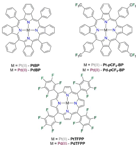
Fig. 1 The chemical structures of the Pt(II) and Pd(II) benzoporphyrin luminophores used in this study. **PtTFPP** and **PdTFPP** are the standard PSP luminophores and are the reference compounds in this study.
