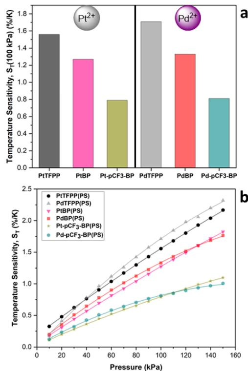
Fig. 6 (a) The  $S_T$  at 100 kPa,  $S_T(100\text{ kPa})$  for the polystyrene-based PSPs. (b) The change in  $S_T$  with pressure for **PtTFPP**, **PdTFPP**, **PtBP**, **PdBp**, **Pt-*p*CF<sub>3</sub>-BP** and **Pd-*p*CF<sub>3</sub>-BP** polystyrene-based PSPs. The data for **PtTFPP** and **PdTFPP** is previously published.<sup>33</sup>
