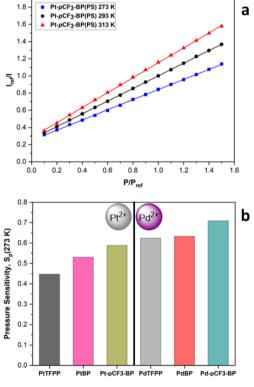
Fig. 5 (a) The modified Stern–Volmer calibrated luminescence response to pressure with associated linear first for Pt-pCF<sub>3</sub>-BP(PS) at 273 K ( $R^2 = 1$ ), 293 K ( $R^2 = 1$ ) and 313 K ( $R^2 = 1$ ). (b) The pressure sensitivity at 273 K,  $S_p$  (273 K), for the porphyrin polystyrene PSPs. The  $S_p$  is calculated using the linear form of the modified Stern–Volmer (eqn S(1)†). The data for PtTFPP and PdTFPP is previously published.<sup>33</sup>
