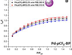
Fig. 7 The modified Stern–Volmer calibrated luminescent response to pressure with 2nd order polynomial fits (eqn S(2)†) at 273 K, 293 K and 313 K for (a) Pt-pCF<sub>3</sub>-BP(3.2% w/w FIB) (average  $R^2=0.995$ ). (b) Pd-pCF<sub>3</sub>-BP(3.2% w/w FIB) (average  $R^2=0.980$ ). The average  $R^2$  is across the fits for the three temperatures.
