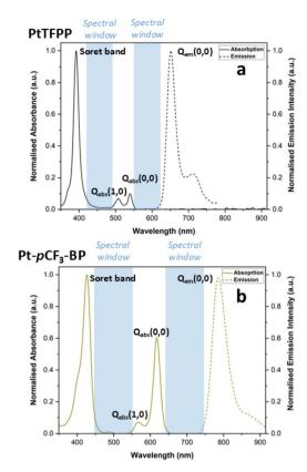
Fig. 3 The normalised absorption and emission spectra of (a) PtTFPP and (b) Pt-pCF<sub>3</sub>-BP showing the 'spectral windows' where a secondary luminophore's emission spectrum could viably occur.
