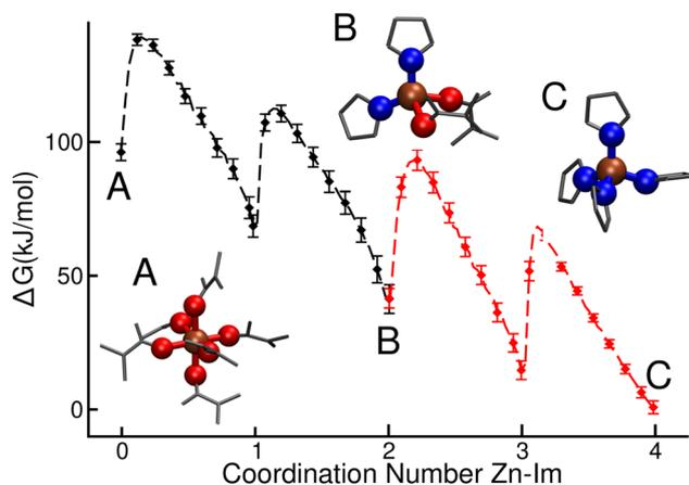
Fig. 2 Free energy as a function of  $n_{\text{Zn-Im}}$  for the full process involving reactions (I) (black curve) and (II) (red curve). Both curves were aligned to match in the common state (labelled as B). The zero of free energy was arbitrarily assigned to the C species. Representative snapshots of the states A, B and C are also shown.
