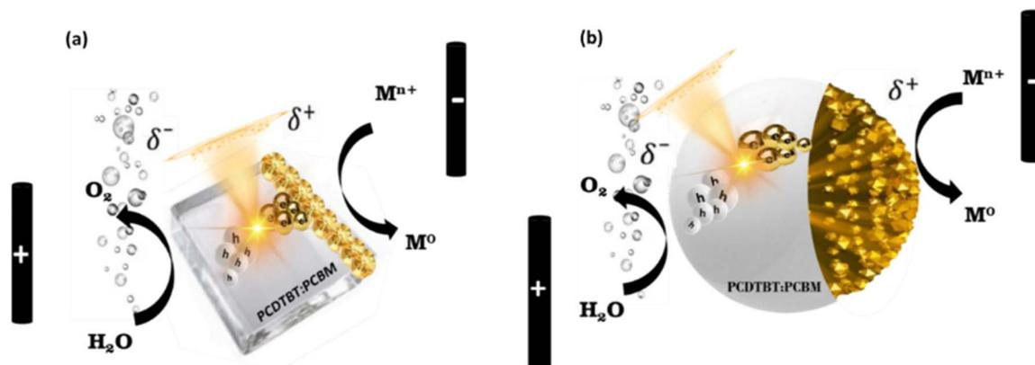
Scheme 1 Scheme of bipolar metal deposition on (a) a PCDTBT:PC<sub>61</sub>BM thin film and (b) a PCDTBT:PC<sub>61</sub>BM particle.
