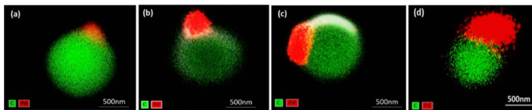
Fig. 5 EDS mapping (C: green; Pd: red) of asymmetric deposits of palladium on PCDTBT:PC<sub>61</sub>BM particles by simultaneous exposure to light and an electric field of 20 kV m<sup>-1</sup> in a solution containing 1 mM of PdSO<sub>4</sub> for different deposition times (a) 30 s, (b) 60 s (c) 2 min and (d) 4 min.
