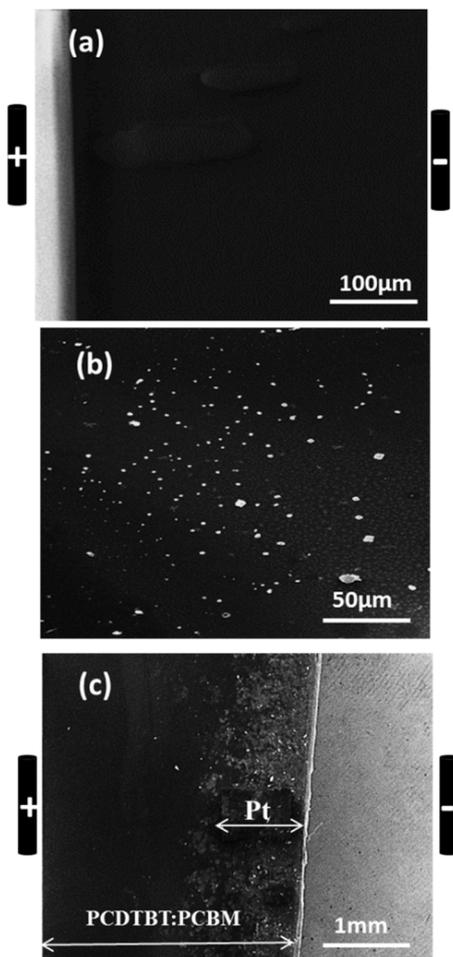
Fig. 1 SEM images of PCDTBT:PC<sub>61</sub>BM thin films after exposition (a) to only an external electric field, (b) only to light and (c) to light and an electric field of 2.8 kV m<sup>-1</sup> for 2 min in the presence of an aqueous solution of 1 mM H<sub>2</sub>PtCl<sub>6</sub>.
