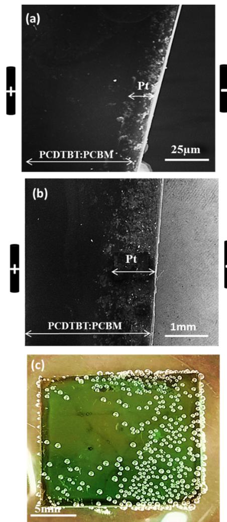
Fig. 2 SEM images of the asymmetric platinum deposit on a thin film of PCDTBT:PC<sub>61</sub>BM after simultaneous application of light (62 mW cm<sup>-2</sup>) and an electric field of (a) 10 kV m<sup>-1</sup>, (b) 2.8 kV m<sup>-1</sup> (c) photograph of a hybrid film of Pt/PCDTBT:PC<sub>61</sub>BM, synthesized at 0.7 kV m<sup>-1</sup>, during photocatalytic water splitting, indicating the asymmetric reactivity by the inhomogeneous distribution of hydrogen bubbles.
