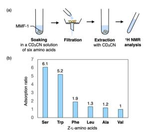
Fig. 5 Selective separation experiment of Z-protected amino acids. (a) Schematic of the experiment. (b) Adsorption ratios of the six residues in MMF-1 estimated by <sup>1</sup>H NMR analysis of the extract.
