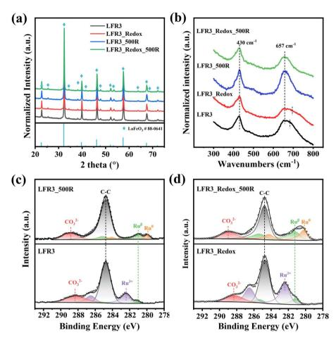
Fig. 1 (a) XRD patterns (blue diamonds are the position of orthorhombic LaFeO $_3$ ) and (b) Raman of the Ru-incorporated samples LFR3\_LFR3\_Redox and Ru-exsolved samples LFR3\_Soor, LFR3\_Redox\_500R. Fitted C 1s + Ru 3d ex situ XPS spectra of (c) LFR3, LFR3\_500R and (d) high-temperature redox treated samples LFR3\_Redox\_and LFR3\_Redox\_500R.
