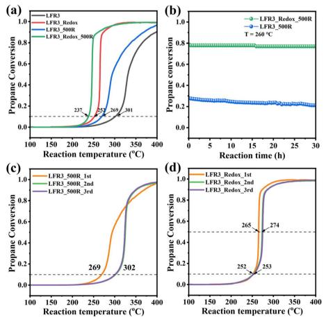
Fig. 5 (a) The activity of Ru-containing perovskites in the propane combustion reaction (1 vol%  $C_3H_8$ , 10 vol%  $O_2$  and 89 vol%  $N_2$  at a total flow rate of 100 sscm), (b) the long-term stability of LFR3\_500R and LFR3\_Redox\_500R at 260 °C. Three consecutive activity tests of (c) LFR3\_500R and (d) LFR3\_Redox\_500R.
