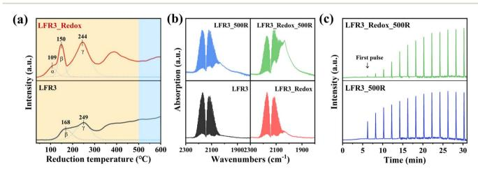
Fig. 4 (a)  $H_2$ -TPR profiles of LFR3 and LFR3\_Redox, (b) CO-DRIFTS of Ru-containing samples that collected in 2 vol% CO/Ar at room temperature, (c) CO pulse results of LFR3\_500R and LFR3\_Redox\_500R.
