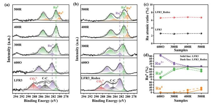
Fig. 2 Fitted C 1s + Ru 3d NAP-XPS of (a) the as-loaded LFR3 and (b) LFR3\_Redox, carbon elimination after oxygen pretreatment at 0.5 mbar  $O_2$  and 600 °C for 1 h (600O) and various reduction treatment at different temperatures (300 °C, 400 °C and 500 °C) under 1 mbar  $H_2$  for 1 h (300R, 400R, 500R). (c) The derived total Ru content and (d) the fraction of Ru in different oxidation states. The fitting parameters are provided in Tables S1 and S2.†
