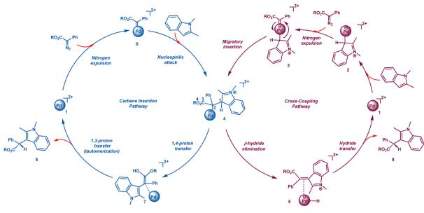
Scheme 2 The conventional carbene insertion and cross coupling catalytic cycles.
