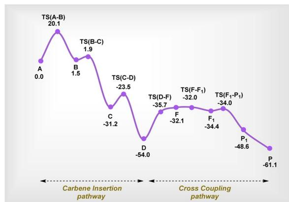
Scheme 8 Free energy profile (kcal mol<sup>-1</sup>) for the lowest energy pathway of carbene insertion into the C3-H bond of indole via the Pd-H intermediate at the SMD(DCM)/DLPNO-CCSD(T)/def2-TZVP//B3LYP-D3/6-31G(d,p),LANL2DZ(Pd) level of theory.
