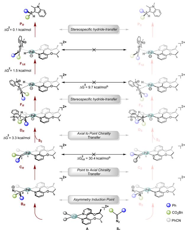
**Scheme 10** Plausible stereochemical model from theoretical calculations.<sup>a</sup> <sup>a</sup>Subscripts *R/S* refer to the stereochemistry of the final product being formed in that pathway and not the stereochemistry of the intermediates being considered. The activation free energy barriers are with respect to the preceding intermediates. <sup>b</sup>Corresponding TSs are given in Fig. S9 of the ESI.†
