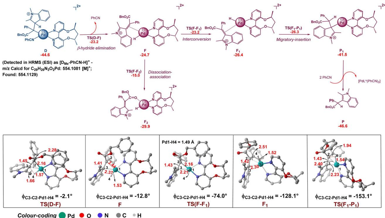
Scheme 7 Formation of alkylated indole via the Pd–H pathway starting from metal ylide **D**. Optimized geometries are given for TSs with distances in Å. Relative free energies are given in kcal mol<sup>-1</sup>. For the TS geometries, hydrogens are removed for clarity.
