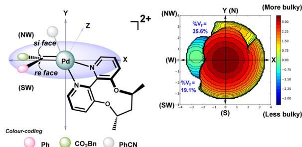
**Fig. 5** Steric map showing percentage free volume (%*V<sub>f</sub>*) available in metallocarbene **C<sub>R</sub>** calculated using SambVca 2.1.<sup>44</sup>
