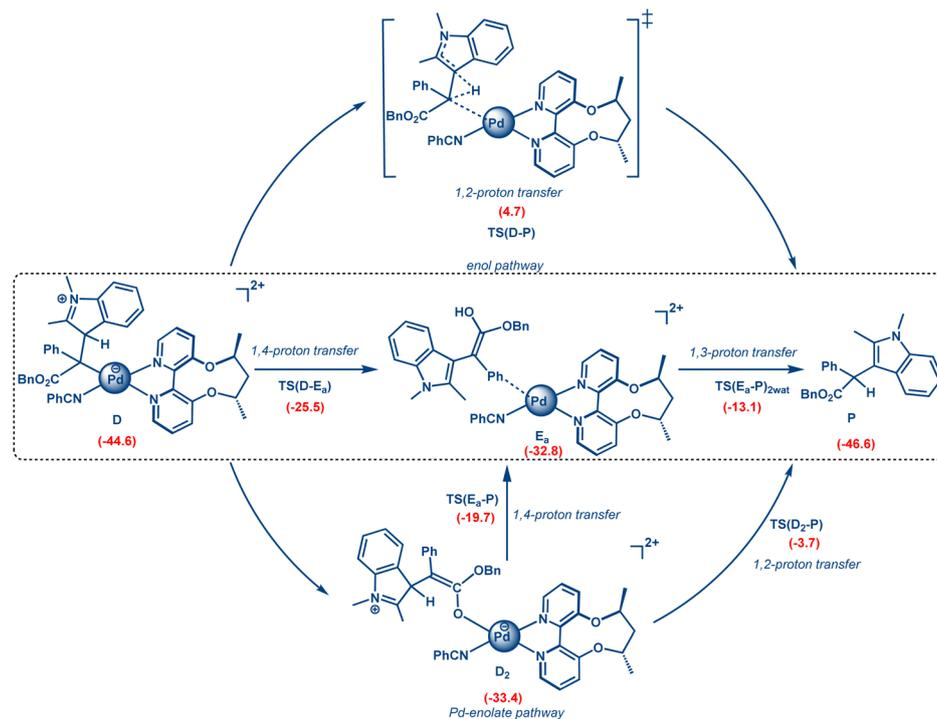
**Scheme 4** Formation of alkylated indole products via 1,2-proton transfer, metal–enol and metal–enolate pathways. The relative free energies (kcal mol<sup>-1</sup>) are given in parentheses at the SMD(DCM)/B3LYP-D3/6-311+G(d,p),LANL2DZ(Pd)//B3LYP-D3/6-31G(d,p),LANL2DZ(Pd) level of theory for the formation of alkylated product P from zwitterion D via the enol pathway.
