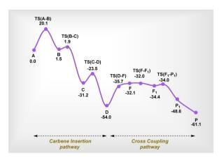
Scheme 8 Free energy profile (kcal  $mol^{-1}$ ) for the lowest energy pathway of carbene insertion into the C3–H bond of indole via the Pd–H intermediate at the SMD<sub>(DCM)</sub>/DLPNO-CCSD(T)/def2-TZVP//B3LYP-D3/6-31G(d,p),LANL2DZ(Pd) level of theory.
