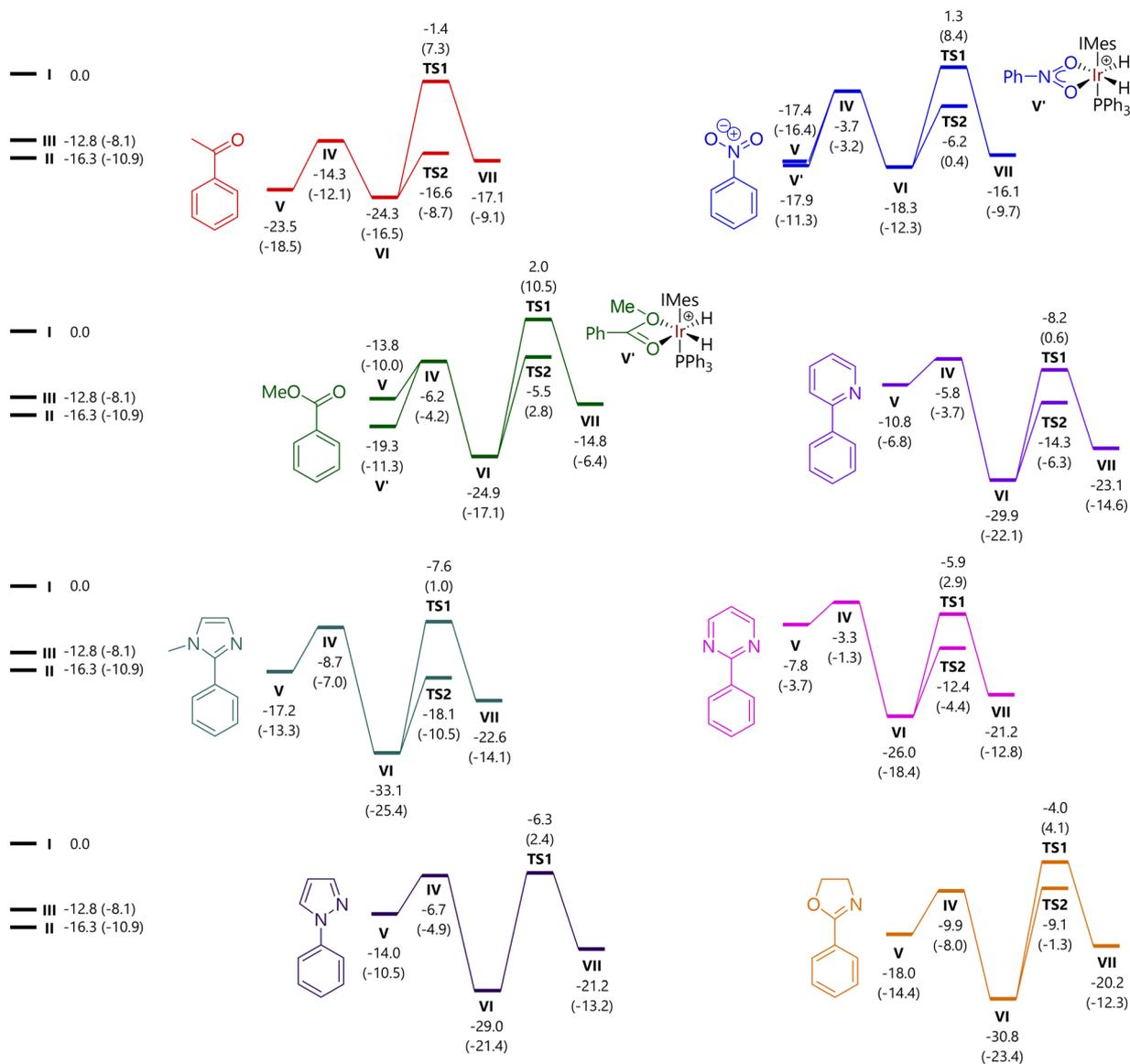
Fig. 5 Free energy profiles for C–H activation reactions at the M06-L/BS2(chloroform) level of theory. Free energies are in kcal mol<sup>-1</sup> relative to structure I and include quasi-harmonic corrections to entropy and enthalpy. Free energies at the M06-L/BS1 (chloroform) level of theory are provided in parentheses.
