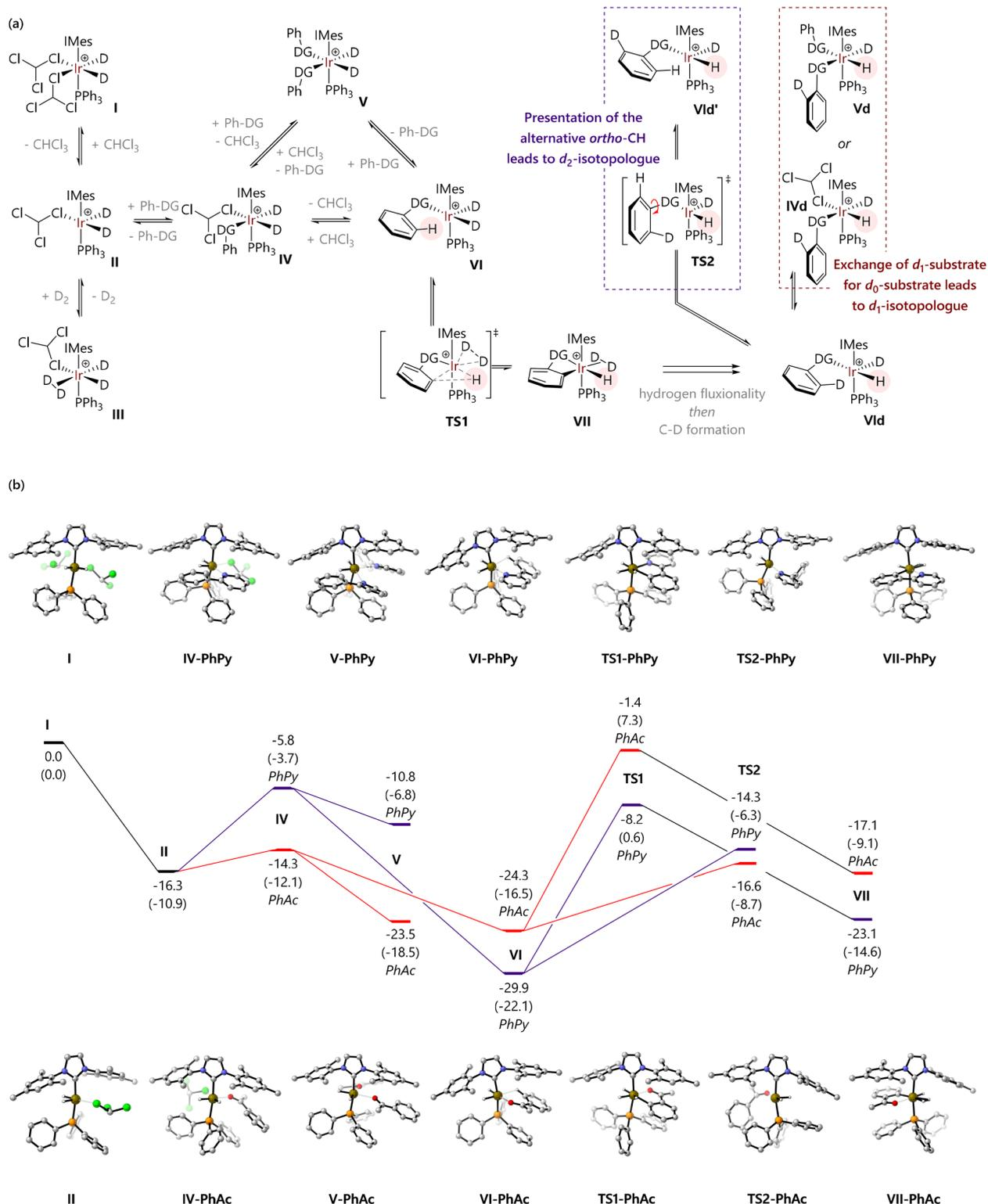
Fig. 3 (a) Reaction mechanisms for the hydrogen isotope reactions studied in this work. (b) Free energy profiles for the reactions of 2-phenylpyridine and acetophenone with [Ir(H)<sub>2</sub>(CHCl<sub>3</sub>)(IMes)(PPh<sub>3</sub>)]<sup>+</sup> (I); free energies are quoted in kcal mol<sup>-1</sup> relative to species I at the M06-L/BS2(chloroform) level of theory, with free energies at the M06-L/BS1(chloroform) level of theory quoted in parentheses.
