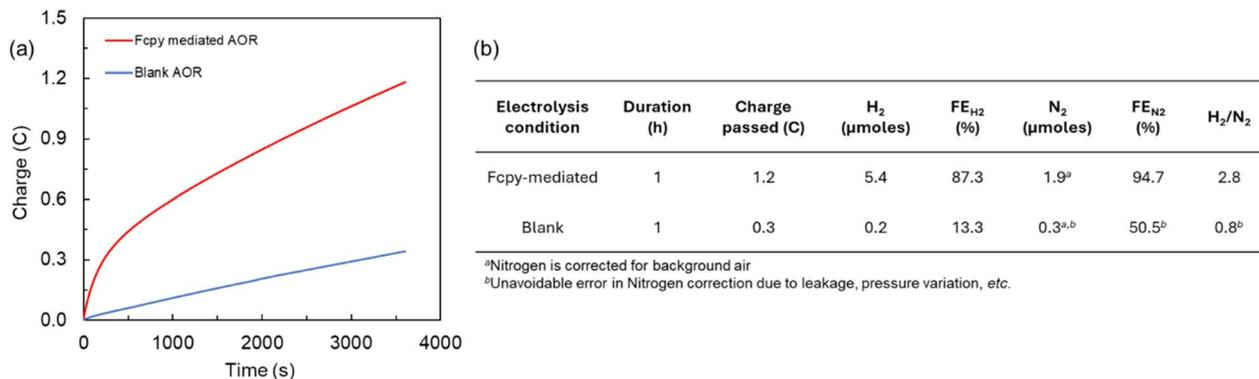
Fig. 3 (a) Constant potential electrolysis at 0.28 V (vs. Fc<sup>+0</sup>) for the same duration without (blue) and with (red) 1 mM Fc-py using 1 × 1 cm<sup>2</sup> carbon-cloth as working electrode. Experimental conditions: 100 mM TBAF as supporting electrolyte in acetonitrile, 3-electrode setup in an undivided cell, 298 K; (b) summary of product quantification results after electrolysis with an average of three measurements.
