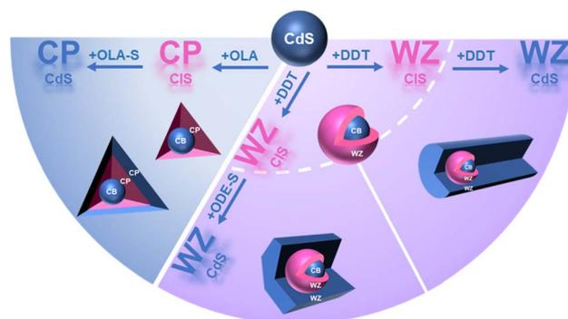
Scheme 2 The formation process of quantum well structures.
