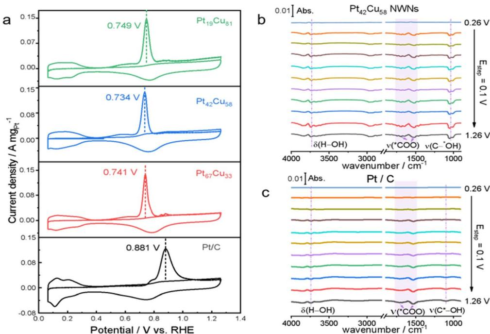
Fig. 4 (a) CO stripping tests of Pt<sub>x</sub>Cu<sub>y</sub> NWNs and commercial Pt/C. (b) Electrochemical *in situ* ATR-FTIR spectrum of the MOR on Pt<sub>42</sub>Cu<sub>58</sub> NWNs and (c) Pt/C.
