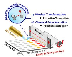
Fig. 1 Concept of array-to-array (reactants-to-products) transfer using DESI for high-throughput small-scale synthesis.
