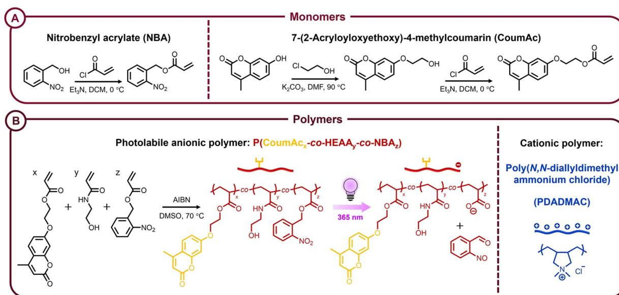
Fig. 2 Reaction schemes for (A) the preparation of the monomer *o*-nitrobenzyl acrylate (NBA) and 7-(2-acryloyloxyethoxy)-4-methylcoumarin (CoumAc) and (B) the conventional radical polymerization of CoumAc, *N*-hydroxyethyl acrylamide (HEAA), and NBA to obtain photolabile polymers P(CoumAc<sub>*x*</sub>-*co*-HEAA<sub>*y*</sub>-*co*-NBA<sub>*z*</sub>).
