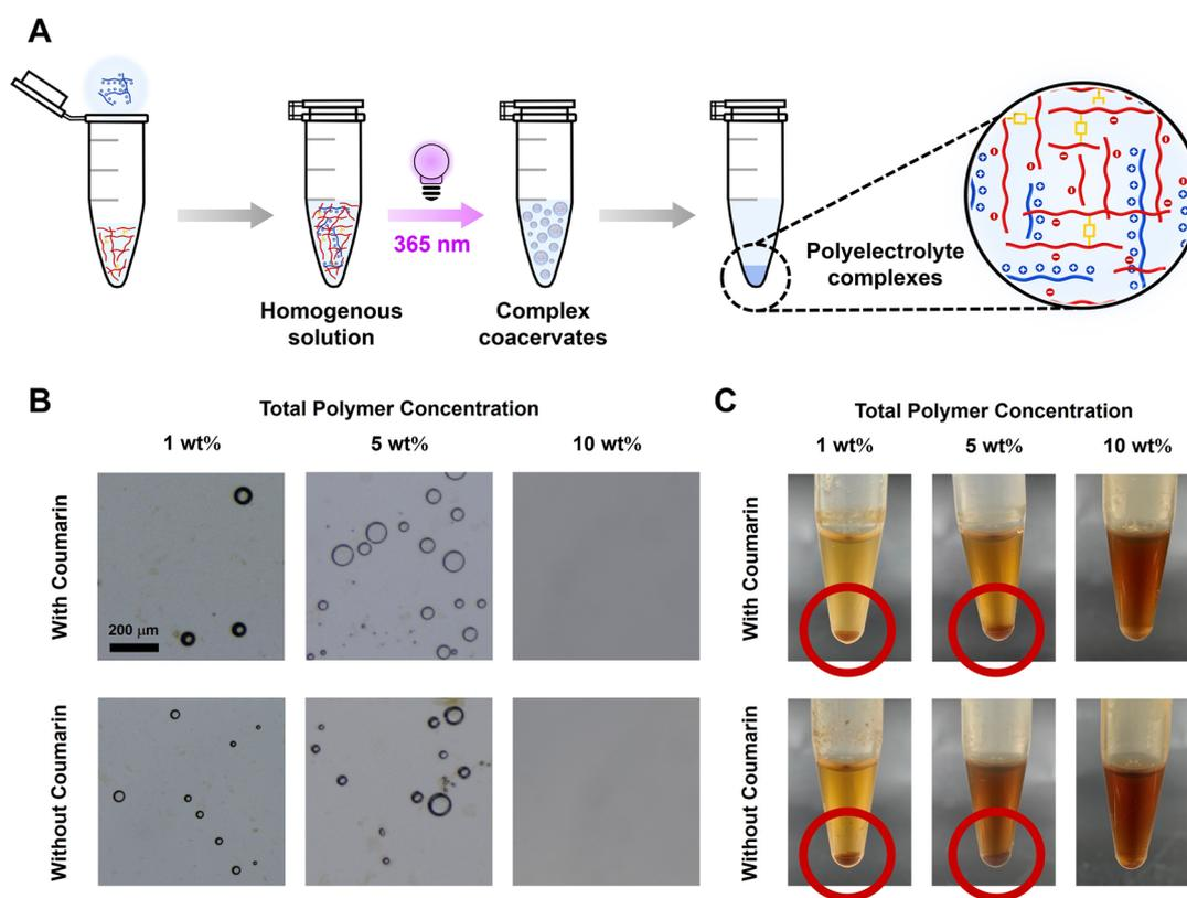
Fig. 4 (A) Schematic representation of the preparation of polyelectrolyte complexes. (B) Optical micrographs and (C) photographs of polyelectrolyte complexes of P(CoumAc<sub>0.03</sub>-*co*-HEAA<sub>0.87</sub>-*co*-NBA<sub>0.10</sub>) or P(HEAA<sub>0.90</sub>-*co*-NBA<sub>0.10</sub>) with PDADMAC under different polyelectrolyte concentrations.
