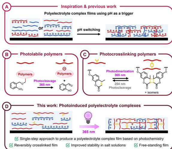
Fig. 1 (A) Previous work demonstrating the preparation of polyelectrolyte complex films using pH as a trigger. Focus on concepts of (B) photolabile polymers containing *o*-nitrobenzyl groups and (C) photocrosslinking polymers containing coumarin groups. (D) This work, wherein polyelectrolyte complexes with reversible crosslinking is achieved using light as a trigger.
