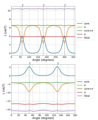
Fig. 3 The angular dependence of the contributions of the core, valence  $\sigma$ , and  $\pi$  orbitals of  $C_3H_3^+$  (top) and of cyclobutadiene (bottom). The MIRC strengths of  $C_3H_3^+$  were calculated using the def2-QZVP basis sets to show that the divergence is smaller when using larger basis sets. The positions of the nuclei are indicated by the vertical dashed lines.
