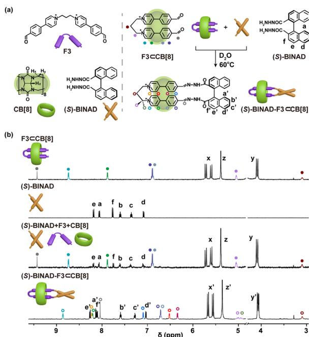
Fig. 2 One-pot synthesis of the chiral ring-in-ring complex. (a) Schematic representation of precursors used for the synthesis of the chiral ring-in-ring complex, (S)-BINAD- $F3 \subset CB[8]$ . (b)  $^1H$  NMR spectra (500 MHz,  $D_2O$ , 298 K) of  $F3 \subset CB[8]$ , (S)-BINAD, and a mixture of (S)-BINAD,  $F3$ , and  $CB[8]$  before and after incubation for 5 hours (from top to bottom). Bromine counterions are omitted for clarity.
