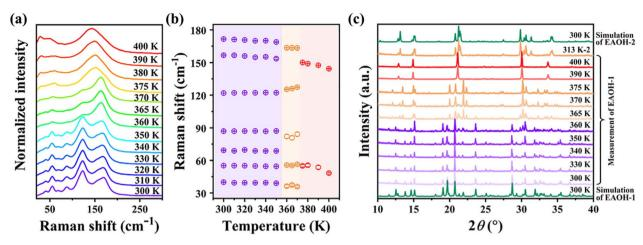
Fig. 2 (a) Selected temperature-dependent Raman spectra of EAOH-1 in the low wavenumber region on heating. (b) Temperature dependence of Raman peaks in (a) fitted with the Lorenz function. (c) The variable-temperature powder X-ray diffraction patterns of compound EAOH-1 and simulated powder X-ray diffraction patterns of compounds EAOH-1 and EAOH-2 at 300 K.
