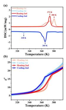
Fig. 1 (a) DSC curves of EAOH-1 in two heating-cooling cycles. (b) Temperature-dependent real part  $(\varepsilon')$  of the dielectric constant of EAOH-1 at 1 MHz in two heating-cooling cycles.
