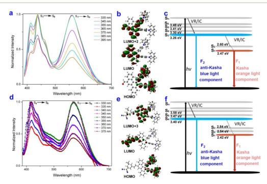
Fig. 1 Anti-Kasha dual-emission characteristics of  $\bf 6u$  and  $\bf 6w$ . (a), (d) Excitation-wavelength-dependent fluorescence spectra of  $\bf 6u$  (0.25  $\mu$ M in DCM) and  $\bf 6w$  (2.4  $\mu$ M in toluene). (b) and (e) Molecular orbitals of the S<sub>0</sub>, S<sub>1</sub>, S<sub>3</sub>, or S<sub>4</sub> states of  $\bf 6u$  and  $\bf 6w$ ; (c) and (f) Jablonski diagram illustrating the anti-Kasha dual-emission mechanism of  $\bf 6u$  and  $\bf 6w$ .
