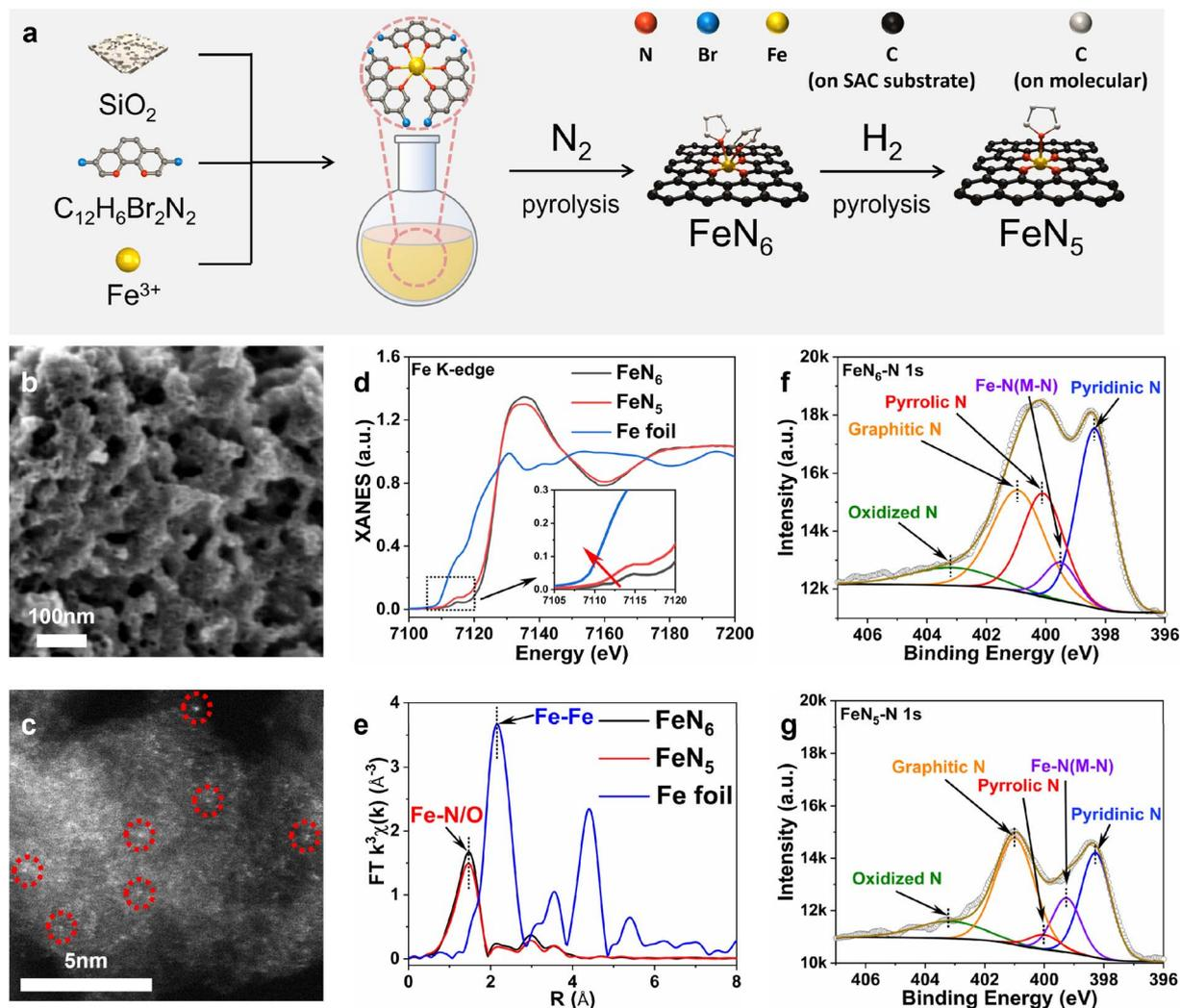
Fig. 1 (a) Schematic illustration of the hard template method for preparing FeN<sub>6</sub> and FeN<sub>5</sub>. (b) SEM image of FeN<sub>6</sub>. (c) AC-HAADF-STEM image of FeN<sub>6</sub> (red circles are the Fe single atom sites). (d) The Fe K-edge XANES spectra. (e) The Fe K-edge FT-EXAFS spectra. (f) The N spectrum of FeN<sub>6</sub>. (g) The N spectrum of FeN<sub>5</sub>.
