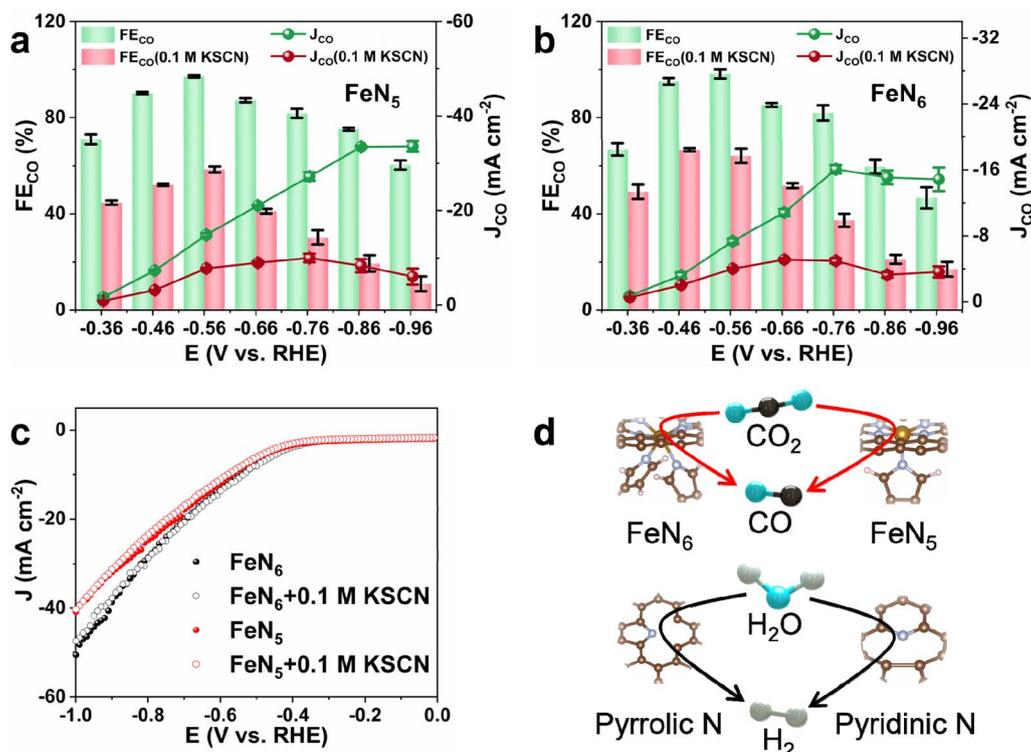
Fig. 3 Catalytic performance of (a) FeN<sub>6</sub> and (b) FeN<sub>5</sub> with (0.4 M KHCO<sub>3</sub> + 0.1 M KSCN) and without 0.1 M KSCN (0.5 M KHCO<sub>3</sub>). (c) The LSV curves of FeN<sub>5</sub> and FeN<sub>6</sub> in an Ar atmosphere with and without 0.1 M KSCN. (d) Schematic illustration of reaction sites in Fe SACs.
