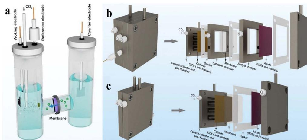
Fig. 2 Diagram of different types of eCO<sub>2</sub>RR electrolytic cells. (a) H-type cell (b) flow cell (c) MEA. (a–c) are reproduced from ref. 59 with permission from Springer Nature Link, copyright 2023.
