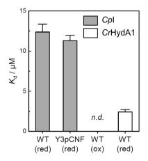
Fig. 6 Microscale thermophoresis. Dissociation constants ( $K_d$ ) of the CpFd:CpI (WT) and Y3pCNF-CpFd:CpI complex under reducing or oxidizing conditions (red/ox). Under oxidizing conditions in the absence of dithionite, an interaction between CpFd:CpI was not detected (n.d.). The open bar depicts the  $K_d$  of the CpFd:CrHydA1 complex under reducing conditions. See Fig. S7† for the titration curves and additional data.
