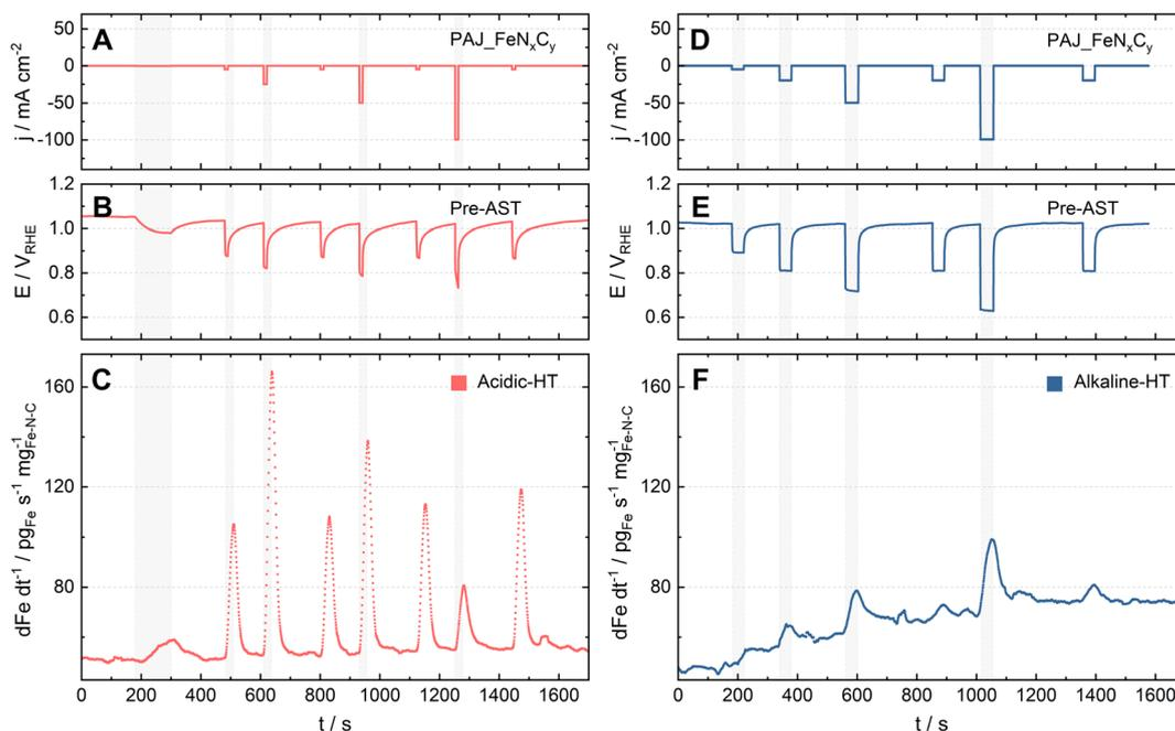
Fig. 2 Online GDE-ICP-MS results during the pre-AST measurements for PAJ\_FeN<sub>x</sub>C<sub>y</sub> (A–C) in 0.1 M HClO<sub>4</sub> at 70 ± 6 °C (Acidic-HT) and (D–F) in 0.1 M NaOH at HT (Alkaline-HT). (A & D) The current density profiles. (B & E) The potential profiles. (C & F) The corresponding online Fe dissolution profiles, which were normalized to the catalyst loading.
