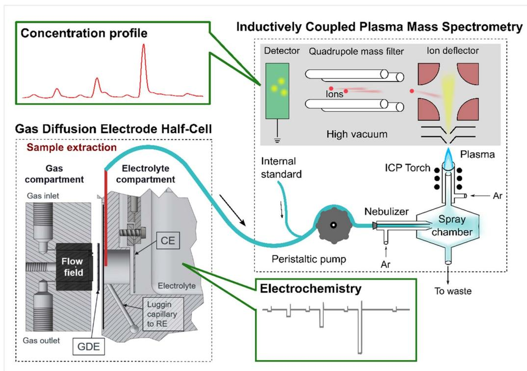
**Scheme 1** An illustration of the gas diffusion electrode (GDE) half-cell coupled to an inductively coupled plasma mass spectrometry (GDE-ICP-MS) setup. The scheme was originally adapted from Fig. S1 in ref. 30 (an open access article). This adapted scheme has been published in our previous work.<sup>15</sup>
