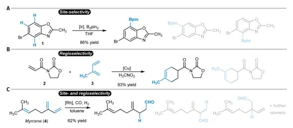
Fig. 1 Site- and regioselectivity of organic reactions. (A) Iridium-catalyzed site-selective borylation that proceeds primarily at one of the three possible  $C_{aromatic}$ -H groups. (B) Copper-catalyzed regioselective Diels-Alder reaction. (C) Rhodium-catalyzed hydroformylation of myrcene with high site- and regioselectivity. In all cases, the main reaction product is shown first, after which additional possible isomers are given half-transparently.
