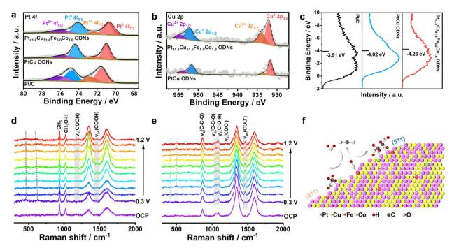
Fig. 5 (a) Pt 4f XPS spectrum. (b) Cu 2p XPS spectrum. (c) Valence band spectra of Pt/C, PtCu ODNs, and  $Pt_{41.8}Cu_{51.6}Fe_{5.0}Co_{1.6}$  ODNs. In situ Raman spectroscopy during the (d) MOR and (e) EGOR. (f) Mechanism of the reaction.
