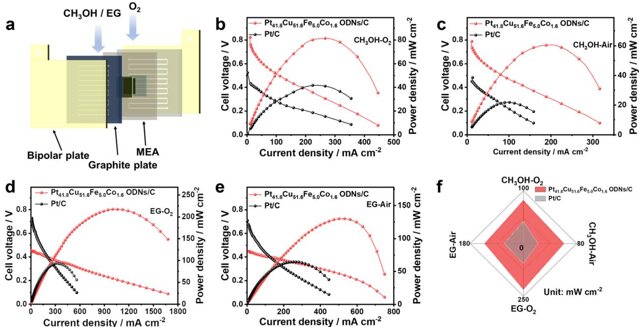
Fig. 4 (a) Structure diagram of the DAFC device. Polarization curves of Pt<sub>41.8</sub>Cu<sub>51.6</sub>Fe<sub>5.0</sub>Co<sub>1.6</sub> ODNs/C and Pt/C in (b) CH<sub>3</sub>OH–O<sub>2</sub> and (c) CH<sub>3</sub>OH–air. Polarization curves of Pt<sub>41.8</sub>Cu<sub>51.6</sub>Fe<sub>5.0</sub>Co<sub>1.6</sub> and Pt/C in (d) EG–O<sub>2</sub> and (e) EG–air. (f) Performance comparison diagram.
