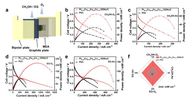
Fig. 4 (a) Structure diagram of the DAFC device. Polarization curves of  $Pt_{41.8}Cu_{51.6}Fe_{5.0}Co_{1.6}$  ODNs/C and Pt/C in (b)  $CH_3OH-O_2$  and (c)  $CH_3OH-air$ . Polarization curves of  $Pt_{41.8}Cu_{51.6}Fe_{5.0}Co_{1.6}$  and Pt/C in (d)  $EG-O_2$  and (e) EG-air. (f) Performance comparison diagram.
