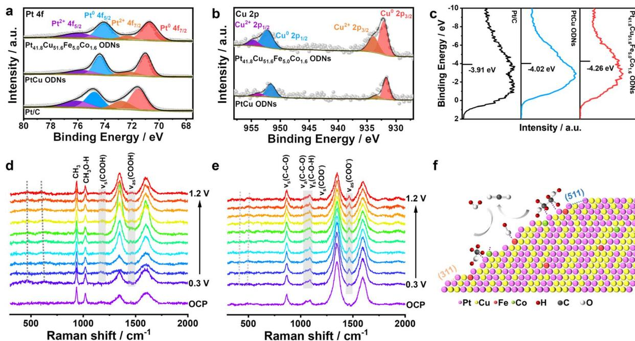
Fig. 5 (a) Pt 4f XPS spectrum. (b) Cu 2p XPS spectrum. (c) Valence band spectra of Pt/C, PtCu ODNs, and Pt<sub>41.8</sub>Cu<sub>51.6</sub>Fe<sub>5.0</sub>Co<sub>1.6</sub> ODNs. *In situ* Raman spectroscopy during the (d) MOR and (e) EGOR. (f) Mechanism of the reaction.
