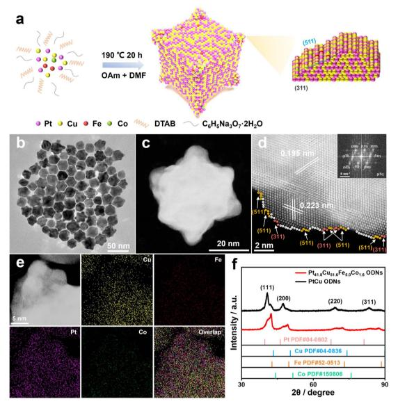
Fig. 1 (a) Schematic diagram of the synthesis of PtCuFeCo ODNs. (b) TEM image of  $Pt_{41.8}Cu_{51.6}Fe_{5.0}Co_{1.6}$  ODNs. (c) HAADF-STEM image of  $Pt_{41.8}Cu_{51.6}Fe_{5.0}Co_{1.6}$  ODNs. (d) AC-HAADF-STEM image of  $Pt_{41.8}Cu_{51.6}Fe_{5.0}Co_{1.6}$  ODNs, and the inset shows the corresponding FFT image. (e) High-resolution elemental mapping images of a single  $Pt_{41.8}Cu_{51.6}Fe_{5.0}Co_{1.6}$  ODN. (f) PXRD pattern of  $Pt_{41.8}Cu_{51.6}Fe_{5.0}Co_{1.6}$  and PtCu ODNs.
