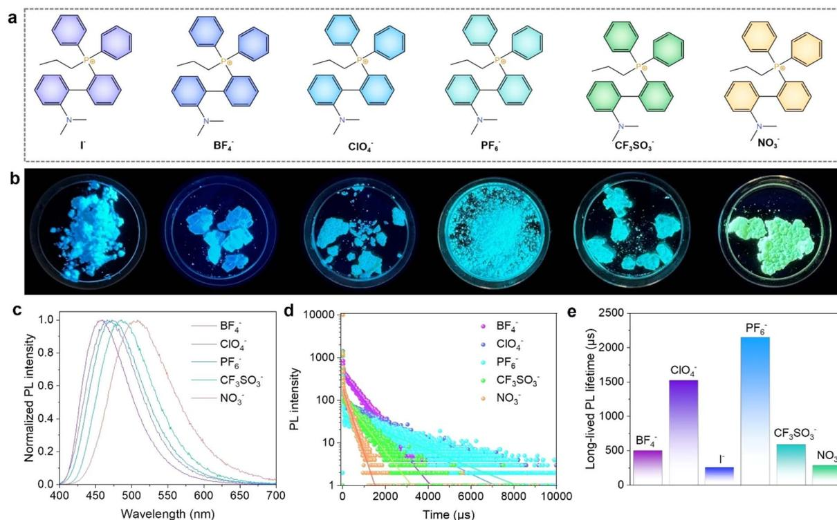
Fig. 2 Role of counter anions. (a) Structures of C3-X with different counter anions. (b) Photographs and (c) PL spectra of C3-X under 365 nm UV light. (d) TRPL decay curves of C3-X at 300 K. (e) Long-lived PL lifetimes of C3-X with different anions.
