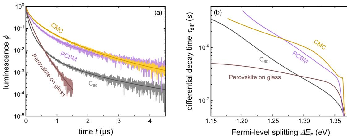
Fig. 15 (a) Tr-PL measurements of three different samples with the layer stack Me-4PACz/triple-cation perovskite/ETL, where the ETL is PCBM, CMC, or C<sub>60</sub>. Furthermore, the tr-PL decay of the perovskite film on glass is presented as a reference. (b) Differential decay times were calculated from the fitted tr-PL data as a function of Fermi-level splitting. Figure reproduced from ref. 30 under the terms of the CC-BY 4.0 license. © The authors of ref. 30 (2023).
