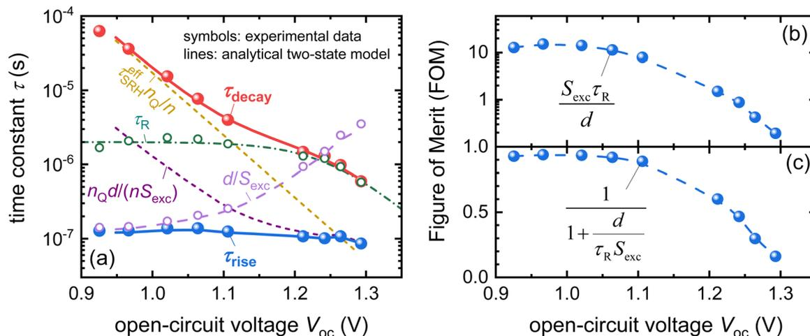
Fig. 17 (a) Time constants extracted from the TPV rise and decay compared with the different terms in eqn (22) and (23) which are shown as dashed or dash-dotted lines. (b) and (c) Figures of merit that follow from the analysis of the rise and decay times shown in panel (a). Reproduced from ref. 17 under the terms of the CC-BY 4.0 license. © The authors of ref. 17 (2023).
