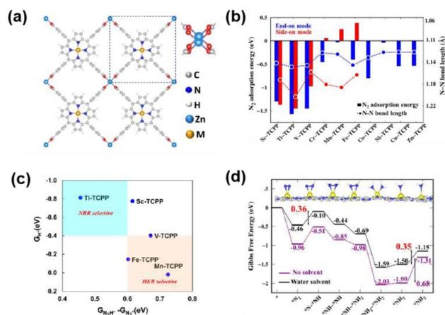
Fig. 6 (a) The optimized structure of M-TCPP 2D-MOFs with the paddlewheel  $\text{Zn}_2(\text{CO}_3)_4$  linker. (b)  $\text{N}_2$  adsorption energies and N–N bond lengths of  $\text{N}_2$  adsorbed in perpendicular and parallel modes in M-TCPP MOFs. (c) NRR selectivity plots of the M-TCPP MOFs with lower limiting potentials. (d) Free energy diagram of the enzymatic NRR on Ti-TCPP. Reproduced with permission from ref. 72. Copyright 2024 American Chemical Society.
