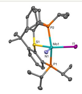
Fig. 4 ORTEP representations (50% probability ellipsoids) of the structure of 1-(N)I determined by X-ray diffraction; hydrogen atoms and PSP t-butyl groups omitted for clarity. Selected bond lengths and angles: Mo1-N1, 1.648; Mo1-S1, 2.353; Mo1-I1, 2.815; Mo1-P1, 2.517; N1-Mo1-S1, 101.12; N1-Mo-I1, 107.26; N1-Mo1-P1, 99.73; N1-Mo1-P2, 99.34; P1-Mo1-P2, 152.55; S1-Mo-I1, 151.62.
