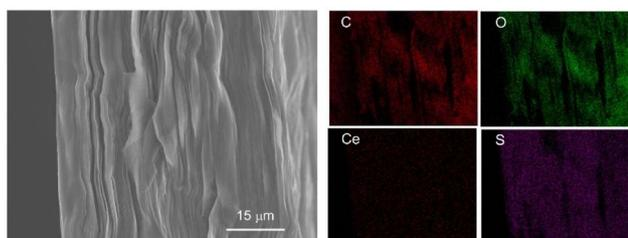
Fig. 2 Cross-sectional SEM image of the graphene oxide (GO) membrane, illustrating a well-organized laminated structure assembled *via* vacuum filtration. The observed stratification indicates the alignment of GO nanosheets, supporting both membrane's stability and selective proton permeability.
