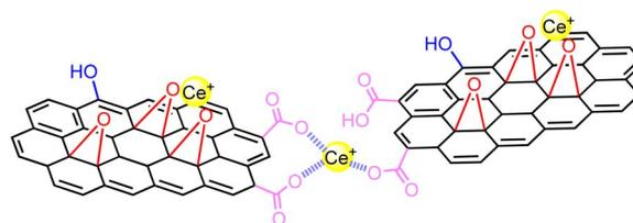
Scheme 1 Schematic representation of Ce<sup>+</sup> grafting in the graphene oxide framework. For clarity, only a few functional groups are shown for clarity.
