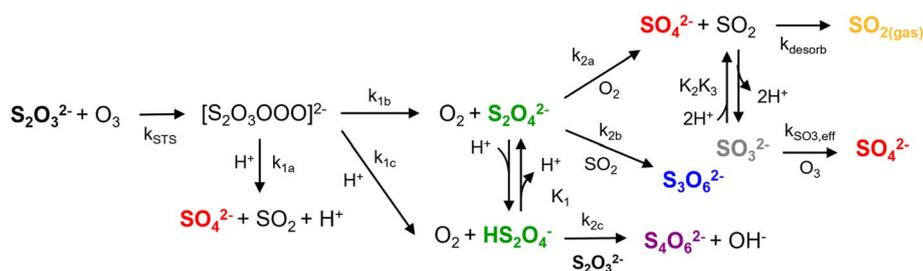
**Scheme 1** Reaction mechanism for the oxidation of aqueous thiosulfate (S<sub>2</sub>O<sub>3</sub><sup>2-</sup>) by ozone (O<sub>3</sub>). Reprinted with permission from Deal, *et al.*<sup>7</sup> Copyright 2024 American Chemical Society.
