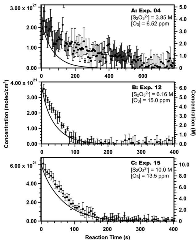
Fig. 6 Select comparisons between data from experiments 4 (A), 12 (B), and 15 (C) in Hsu, *et al.*<sup>9</sup> and the kinetic model (lines). Data with error bars are recreated from ref. 9. See Section S6 in ESI† for all comparisons between model and experiments.
