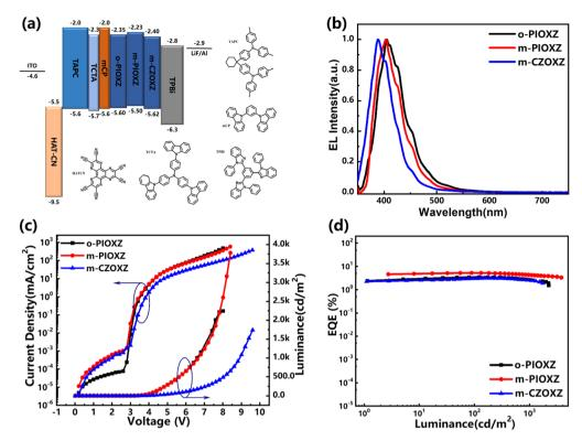
Fig. 7 (a) Energy level diagrams; (b) EL spectra; (c) luminance-voltage-current density curves of non-doped OLEDs; and (d) external quantum efficiency-luminance curves.
