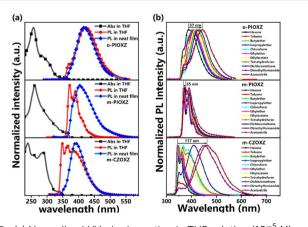
Fig. 3 (a) Normalized UV-vis absorption in THF solution ( $10^{-5}$  M) and normalized PL spectra in THF ( $10^{-5}$  M) and in the film state; (b) normalized PL spectra of the three materials in different solvents with increasing polarity.
