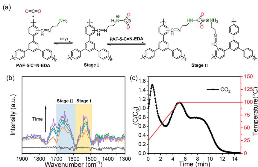
Fig. 5 (a) Chemisorption mechanism of amines and CO<sub>2</sub> under dry conditions; (b) IR absorption spectra of adsorbed species on PAF-5-C=N-EDA at 25 °C taken at different times during CO<sub>2</sub> adsorption; (c) adsorbed phase analysis of PAF-5-C=N-EDA by using Temperature Programmed Desorption (TPD).
