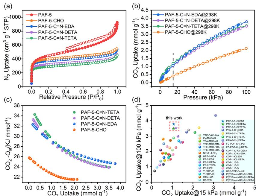
Fig. 3 (a)  $N_2$  uptake at 77 K; (b)  $CO_2$  uptake of PAF-5-CHO and its derivations at 298 K; (c)  $CO_2 -Q_{st}$  of PAF-5-CHO and its derivation; (d) comparison of  $CO_2$  uptake with other amine-functionalized POPs at 15 kPa and 100 kPa.<sup>20,46–57</sup>
