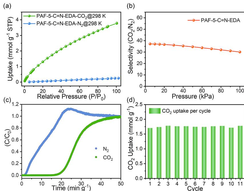
Fig. 4 (a) N<sub>2</sub> and CO<sub>2</sub> uptake of PAF-5-C=N-EDA at 298 K; (b) CO<sub>2</sub>/N<sub>2</sub> selectivity of PAF-5-C=N-EDA; (c) breakthrough curves of PAF-5-C=N-EDA for a CO<sub>2</sub>/N<sub>2</sub> (15 : 85,v/v) gas mixture with a total flow of 10 mL min<sup>-1</sup> at 298 K and 1 bar; (d) CO<sub>2</sub> uptakes of PAF-5-C=N-EDA derived from the breakthrough cycling measurement.
