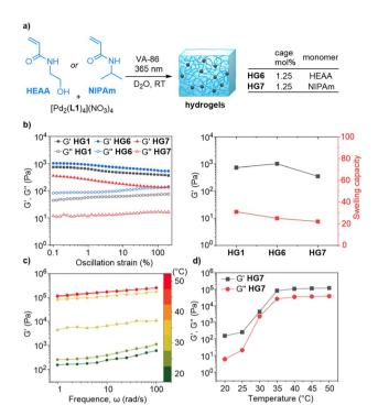
Fig. 4 (a) Synthesis of the hydrogels HG6 and HG7 by photoinitiated copolymerization of HEAA or NIPAm with  $[Pd_2(L1)_4](NO_3)_4$ . (b) Rheological data and swelling capacities of gels based on different monomers (HG1, HG6, and HG7). (c) Storage moduli G' of HG7 as a function of the angular frequency at different temperatures. (d) Storage moduli G' and loss moduli G'' (at 1 rad s<sup>-1</sup>) of HG7 at different temperatures.
