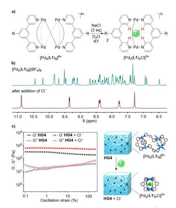
Fig. 5 (a) Chloride-induced rearrangement of  $[Pd_4(L1)_8]^{8+}$  into  $[Pd_2(L1)_4Cl]^{3+}$ . (b)  $^1H$  NMR spectra (400 MHz,  $D_2O$ ) of a solution of  $[Pd_4(L1)_8](BF_4)_8$  in  $D_2O$  before (top) and after chloride-induced rearrangement (bottom). (c) Rheological data of HG4 before and after treatment with chloride.
