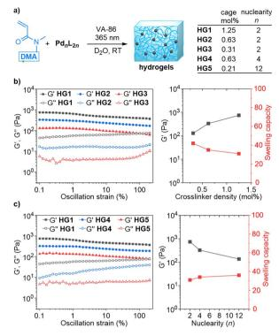
Fig. 3 (a) Synthesis of the hydrogels HG1-HG5 by photoinitiated copolymerization of DMA with [Pd<sub>2</sub>(L1)<sub>4</sub>](NO<sub>3</sub>)<sub>4</sub>, [Pd<sub>4</sub>(L1)<sub>8</sub>](BF<sub>4</sub>)<sub>8</sub>, or  $[Pd_{12}(L2)_{24}](BF_4)_{24}$ . (b) Rheological data and swelling capacities of gels with different crosslinker densities (HG1-HG3). (c) Rheological data and swelling capacities of gels with different cage crosslinks (HG1, HG4, and HG5)
