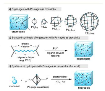
Fig. 1 (a)  $Pd_nL_{2n}$ -type cages with nuclearities ranging from n = 2 to 24 have been used as crosslinks in organogels. (b) The standard synthesis of organogels with Pd-cages as crosslinks. (c) Synthesis of hydrogels by copolymerization of monomers with Pd-cages featuring acrylate side chains (this work)
