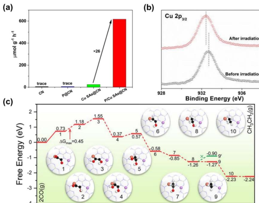
Fig. 7 (a) Photo-driven CO<sub>2</sub>RR generates C<sub>2</sub>H<sub>6</sub> on CN, P@CN, CuSAs@CN and P/Cu SAs@CN. (b) Cu 2p<sub>3/2</sub> over P/Cu SAs@CN before and after light irradiation. (c) Free energy diagram of CO coupling reduction to C<sub>2</sub> products on P/Cu SAs@CN photocatalyst and atomic structure of reaction intermediates.<sup>97</sup> Copyright 2022, Wiley.
