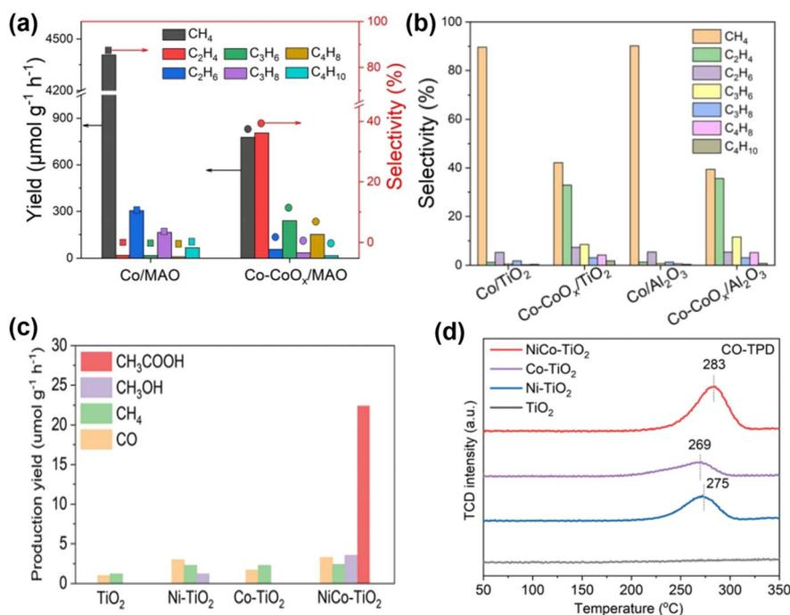
Fig. 6 (a) Product yield and selectivity of CO<sub>2</sub> hydrogenation in a closed gas circulation system. (b) Product selectivity relative to other catalysts.<sup>9</sup> Copyright 2023, Wiley. (c) Yield of CH<sub>3</sub>COOH and other products under UV-visible light irradiation. (d) CO-TPD spectra of NiCo-TiO<sub>2</sub>, Ni-TiO<sub>2</sub>, Co-TiO<sub>2</sub> and TiO<sub>2</sub>.<sup>96</sup> Copyright 2022, Wiley-VCH Verlag.
