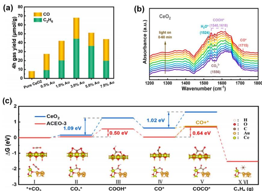
Fig. 10 (a) CO and C<sub>2</sub>H<sub>6</sub> generation rates as a function of Au content; *in situ* FTIR spectra of CO<sub>2</sub> and H<sub>2</sub>O vapor mixtures co-adsorbed on (b) CeO<sub>2</sub>. (c) Reaction pathway for Gibbs free energy calculation of photocatalytic CO<sub>2</sub> reduction.<sup>103</sup> Copyright 2023, Elsevier.
